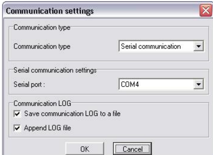
Fig. 25 – Communication Setting Window
