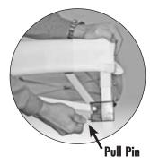
**2.** Release pull pin at each corner by first lifting valance fabric away from slider. With one hand push up on truss near the pull pin, pull the pin out to release. **Note:** It is much easier to release pull pin when the shelter weight has been removed from the pull pin.
