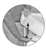
**2.** To engage the Auto Slider® at each corner, first lift the fabric off of the slider, then with one hand hold the top of the leg while pushing up on the slider with the other hand. The pull pin will engage the hole. Pull down the fabric valance over the slider. Repeat on all four corners.
