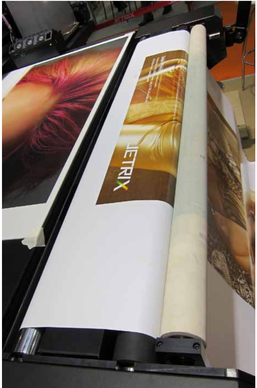
The roll system is totally attached to the chassis of the printer.
