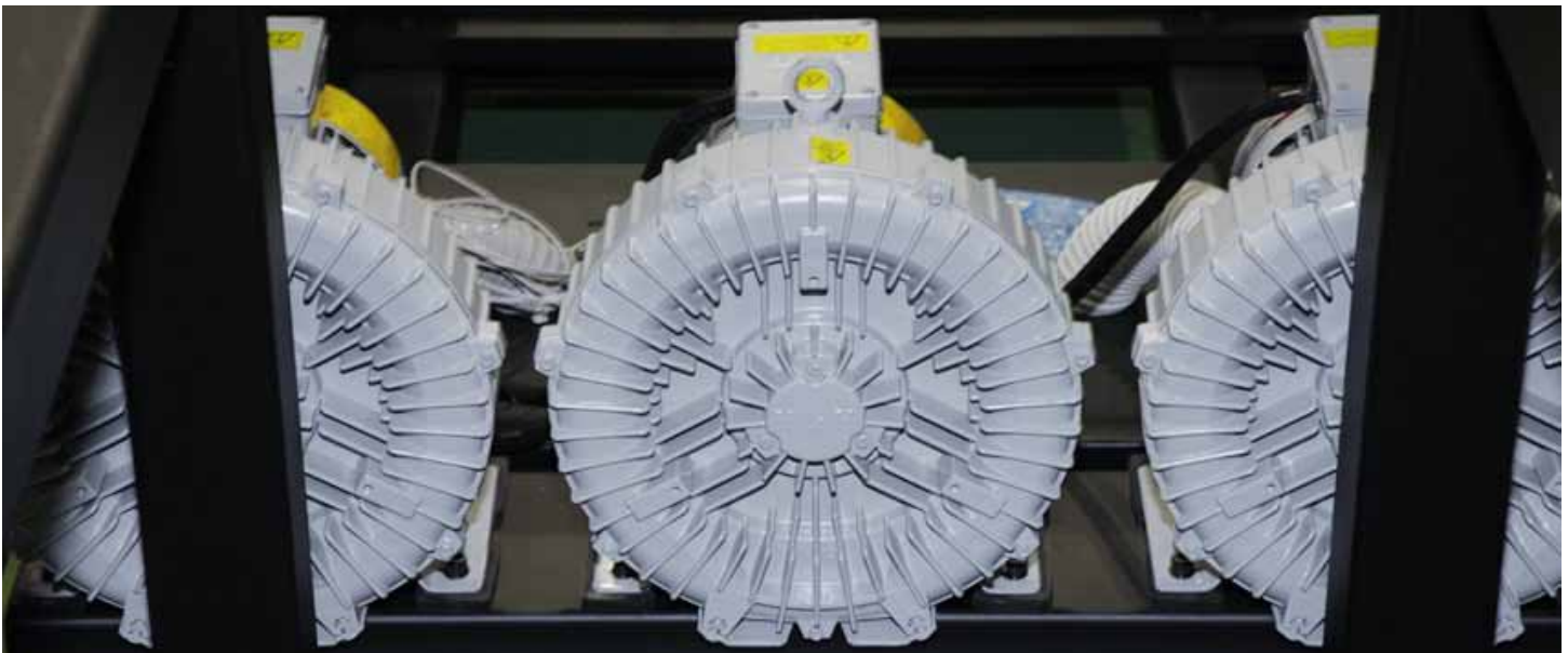
Photograph taken during FLAAR's visit to JETRIX factory. The three vacuum pumps are visible through the printer's framework.
