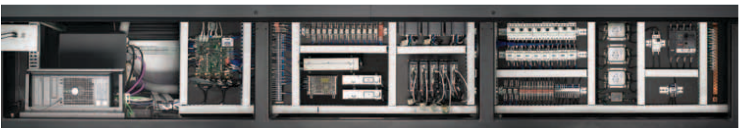
Most of the electronic boards are located at the left side of the printer, including the electronics of the vacuum system.
