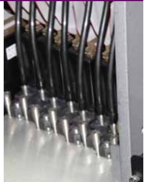
The Konica Minolta 1024 heads produce a swath of 72mm, which is twice the length covered by the previous printhead model, the KM 512.
