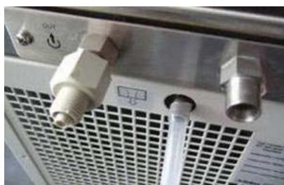
5. Slide a finger nut and olive onto the other end of the coolant hose.
