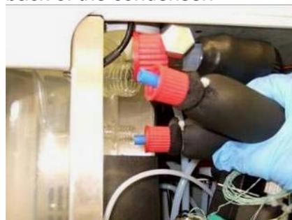
9. Lift and wiggle the glass condenser assembly upwards until clear of the evaporator. Place the glass condenser assembly on a suitable work surface.
