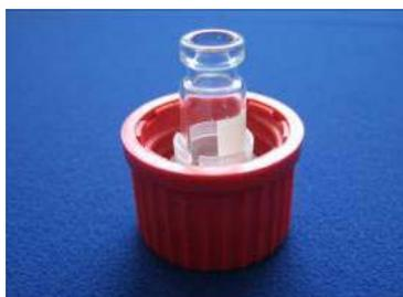
5. Screw a flask onto the vial / cap assembly. Take care to ensure the vial aligns centrally with the vial seal.
