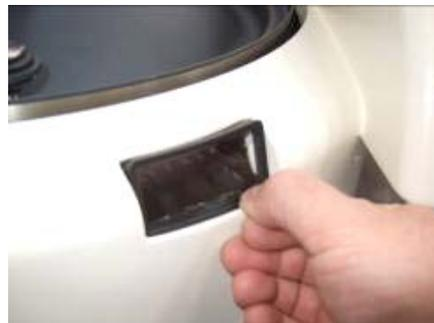
3. Remove the cladding window and wipe clean using non abrasive paper towel or lint free cloth.
