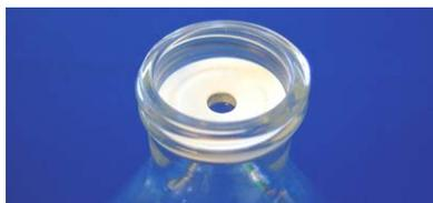
**Note:** Standard **SampleGenie vial seals** are manufactured from low leachable viton. Perfluoroelastomer seals are also available.
