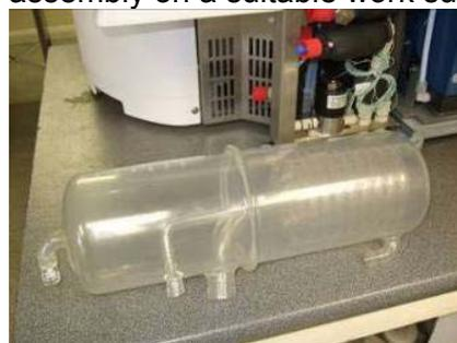
Inspect the glass condenser assembly to ensure it is free from cracks, nicks and other damage. A replacement condenser glass is available as a spare part.
