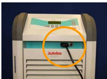
If an alternative re-circulating cooler is used (or if the Julabo re-circulating cooler comms lead is not connected) the coolant temperature will have to be set manually. The optimum coolant supply temperature for each solvent is defined within the appropriate method. To find the appropriate coolant temperature, select **View Method** from the **Method Select** menu, and scroll down to find the **Chiller Set Temp**.
