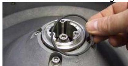
13. Remove the inner lid sealing O ring.
