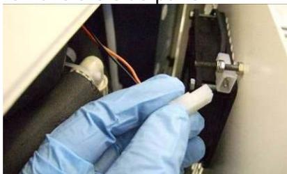
4. Remove the pump tray retaining screw and pull out the pump tray assembly as far as the PTFE hoses will allow.
