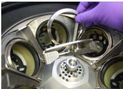
6. Use a flat tool such as a spatula to release the flask adaptor locking tab.
