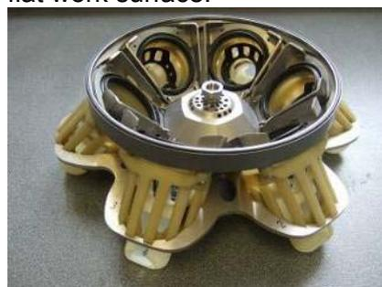
12. Remove the rotor shaft O ring.
