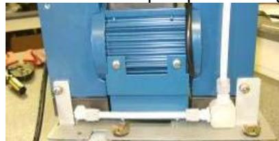
10. Turn the pump around and remove 2x M5 pump mounting screws.
