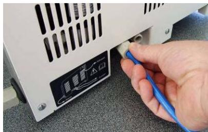
4. Screw a hose adaptor onto the re-circulating cooler **feed** (or **out**) connector.
