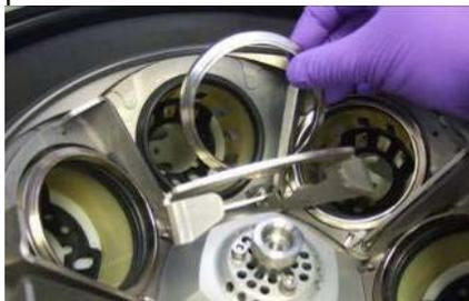
6. Use a flat tool such as a spatula to release the flask adaptor locking tab .
