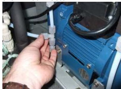
7. Pull the pump tray all the way out and position the pump assembly to one side.
