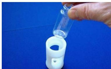
4. Screw an assembled flask, flask collar and collar pad onto the vial adapter.
