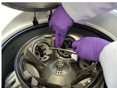
Start at one point, move to the point at 180° (opposite) then the points at 90° and 270°. Then work around the seal until the seal lip is flush with the basket all the way round.
