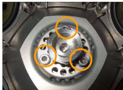
10. Lift the rotor assembly free it from the shaft and away from the evaporator.
