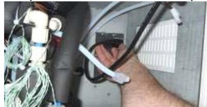
9. Remove 2x M6 pump mounting screws
