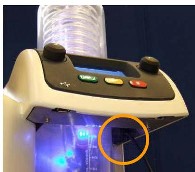
2. Connect the male end of the comms lead to the re-circulating cooler socket located under the re-circulating cooler control panel.
