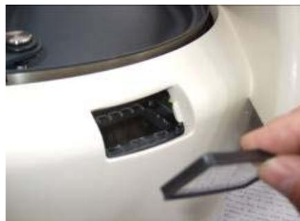
4. The upper side of the chamber window is now accessible for cleaning. Take care to avoid damaging the window heating element (if fitted).
