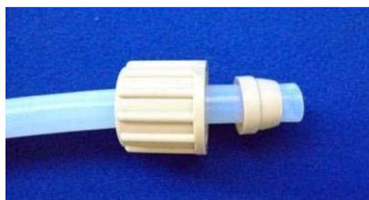
2. Connect the waste solvent drain hose to the waste solvent drain connector. Hold the hose against the solvent drain connector and screw the compression nut onto the spigot until finger tight.
