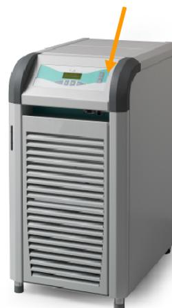
Providing the comms lead is connected and **remote mode** is enabled, the re-circulating cooler starts and displays the current coolant temperature. The evaporator then assumes control of the re-circulating cooler.
