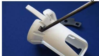
11. Repeat for the other end of the flask cushion. Ensure the cushion is correctly seated in the flask adapter.
