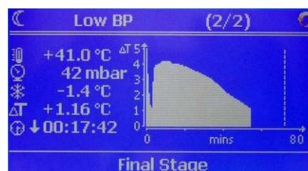
Final drying stage, evaporator running to time
