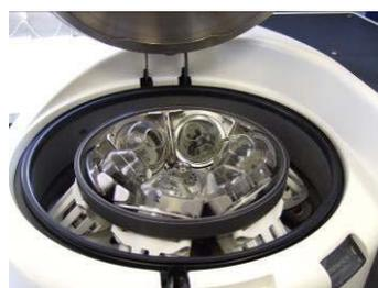
5. Replace the inner lid and secure with the thumb screw. Turn the thumb screw clockwise until light resistance is felt. Tighten by continuing to turn clockwise for a further three quarters of a turn.
