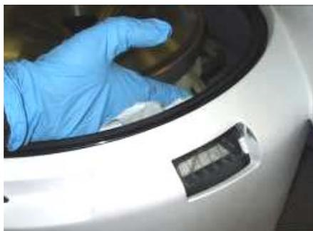
2. Press in the lower edge of the cladding window, the top pops out and the window is released from the cladding aperture.
