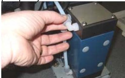
6. Disconnect the plastic hose connector to release the back left PTFE hose from the "T" connector.
