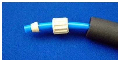
6. Connect the coolant hose to re-circulating cooler **feed** adapter. Hold the coolant hose against the adapter and screw the finger nut onto the adapter until finger tight.
