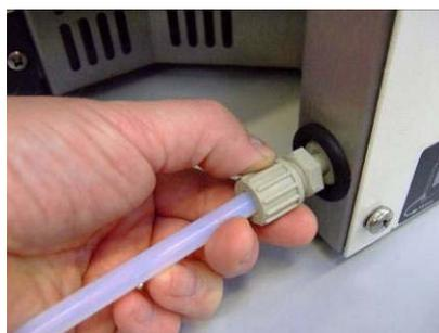
3. Cut the waste solvent drain hose to a suitable length so it may be connected to the waste solvent container.
