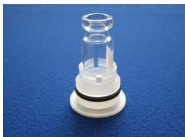
4. Place the assembled vial and vial holder into a **flask cap**.
