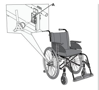
The one arm drive enables you to move the wheel-chair with one hand. Two hand rims are installed on the same wheel. The drive wheel can be fitted on the right or left side.
