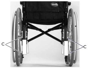
When the drive wheel attachments are mounted (forwards or backwards, see previous page) it is the outer, lower part (C) of the attachments that decides the camber of the rearwheels. The picture illustrates drive wheel attachments that give 0° camber. If the wider part of the attachment had been placed downwards the camber would have been 2° instead.
