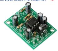
This kit has been developed as a pre-module for a number of audio applications where there is insufficient input signal.
