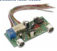
The Velleman Ultrasonic Radar Module is designed for use with security systems, car parking or the detection of objects - in fact any project where an indication of distance is required. The module gives off a buzzing sound when the trget is detected.
