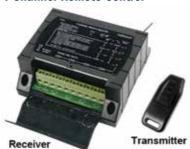
The Velleman 4-Channel Remote Control Module is a mains operated 4-channel RF receiver which can be used as a remote or codelock security transmitter/receiver. Also available is a handheld 4-channel RF transmitterand a desktop RF transmitter.
