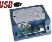
The Velleman USB-Controlled DMX Interface Kit enables you to control DMX lighting fixtures using a PC and USB interface. Test software and DMX Light Player software is included, and a Dynamic Link Library (DLL) is provided to write your own software. The device includes a standalone test function that outputs all 512 channels at a time, with adjustable levels.
