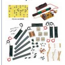
This project offers students a cost-effective way to build an AM tuner that is easy to incorporate into a variety of design situations. The Printed Circuit Board (PCB) can be either purchased ready made, or students can manufacture their own from the mask provided in the notes. Project notes are available for free download at www.rapidonline.com and can be photocopied for class
