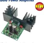
This small amplifier is constructed with a maximum supply capability of 2x 15Wrms (4 $\Omega$ ) of 2x 10Wrms
