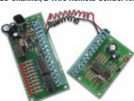
The Velleman 10-Channel, 2-Wire Remote Control Kit allows you to control up to 10 devices using only 2 wires from up to 50 metres away. Inputs can be push-buttons, switches or open collector outputs from another device and the receiver section provides 10 open collector outputs that allow you to control relays directly. Terminal block connectors for all input and output connections are included.
