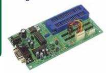
The Velleman PIC Programmer Board can be used to programme a wide range of Microchip PIC microcontrollers and is suitable both for serious industrial applications and by hobbyists in schools and colleges It is available either in kit form or as a pre-assembled module
