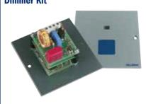
This one channel IR Remote Controlled Light Dimmer Kit from Velleman produces a device that can be set to 1 of 15 transmitter codes. Thanks to its compact design, this kit fits into a standard light switch housing.
