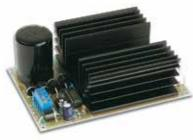
This Velleman Power Supply Kit is meant as an auxiliary or as a permanent power supply for all common Velleman kits based on a stabilised DC voltage between 3 and 30V, provided that the consumption does not exceed 3A, but can also be used for other purposes. By replacing the trimmer with a potentiometer it can even be used as an adjustable power supply unit.
