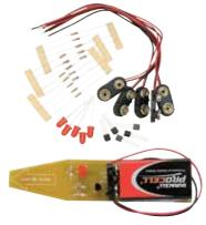
Kits of components to build a functional Moisture Tester that can be used to tell if pot plants require water.
