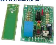
There are times when too much water can be a problem, just as there are occasions when too little can leave you in trouble. The Velleman Liquid Level Controller is the solution. With this kit you can build a device which monitors levels to warn you if your water tank is close to overflowing or running dry. It can indicate Low, Middle and High levels; automatically switch a pump to keep the right fluid level; and if the sensor detects a level which is
