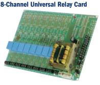
If you want to switch large electric currents using an electronic control and require control isolation at the same time, then this 8-Channel Universal Relay Card from Velleman could be just what you need.
