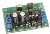
The Velleman Symmetric 1A Power Supply Kit provides a low-cost, compact universal symmetric power supply, ideal for amplifiers or op-amp applications. Just add a suitable transformer and a heatsink and you're ready to go. Trimmers can be replaced by potmeters to allow continuous adjustment of output voltage.
