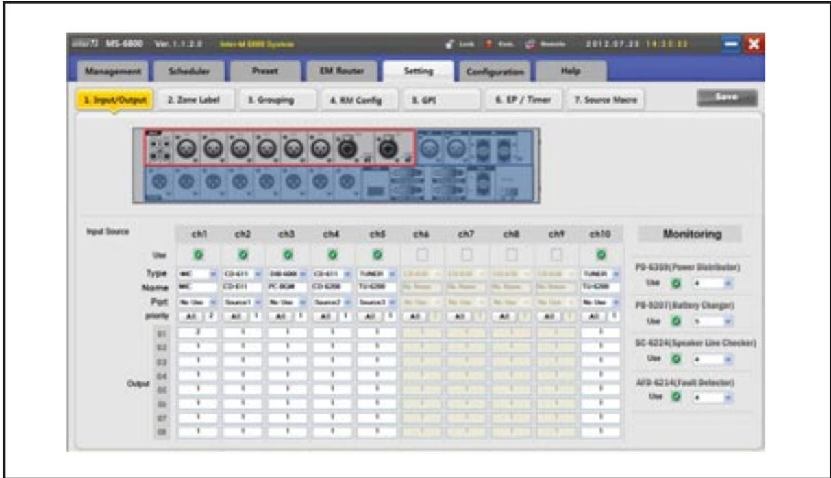
\* Input source setting displays 10 channel lists to the lateral direction and detail setting values for each channel can be set to the vertical direction.
