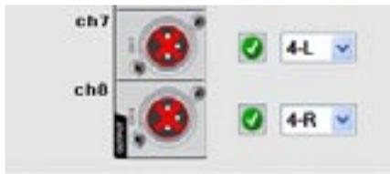
(3) Select output : select the output channel to be broadcasted in 16 zones of ECS-6216MS.
