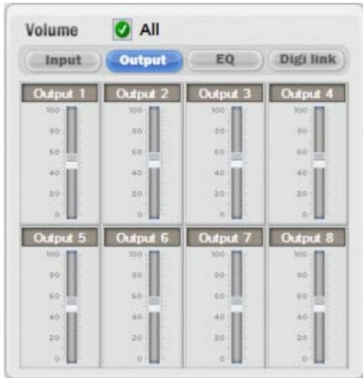
3) Output EQ : controls 8 channel of individual EQ volume of PX-6216
