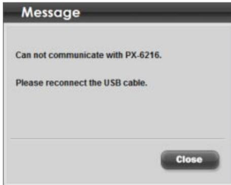
B) If port and PC settings are incorrect in the [Configuration>Port Setting] of the program, it should be reset in the communication port setting [Refer to Page 21]
