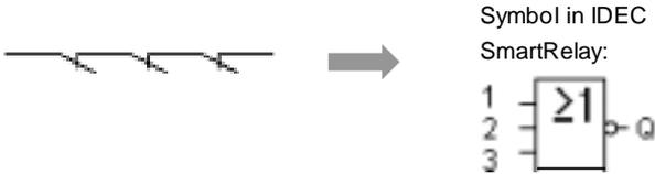
The output status of the NOR is only 1 if all inputs are 0, if switched off. The NOR output is set to 0 at the 0 to 1 transition at one of the inputs. The status of a block input pin which is not connected (x) is: x = 0.
