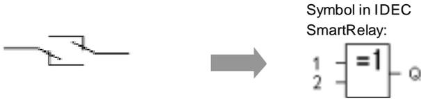
The output status of the XOR is 1 if the inputs are not equivalent.
