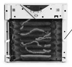
3. Remove the used filter by lifting the pull string.
