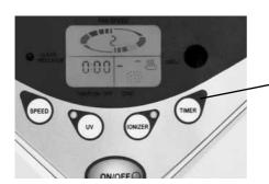
RESET the filter indicator by holding down TIMER while the unit is ON until the clean indicator light disappears.
