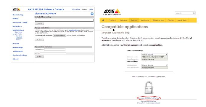
Click in the link on the *Manual Installation* section (ww.axis.com), it will connects to the AXIS license service (<a href="http://www.axis.com/techsup/compatible\_applications/">http://www.axis.com/techsup/compatible\_applications/</a>). Insert the license code and the camera's serial number.
