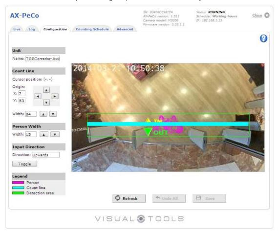
Count Line Configuration. On the left menu, use the arrows in the Count Line section to set up the people traffic line in the image. To define the counting zone use the arrows at the Width option.
