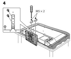
**Warning:** Ensure the power cable is not pinched when attaching the pedestal stand as this could cause an electric shock.
