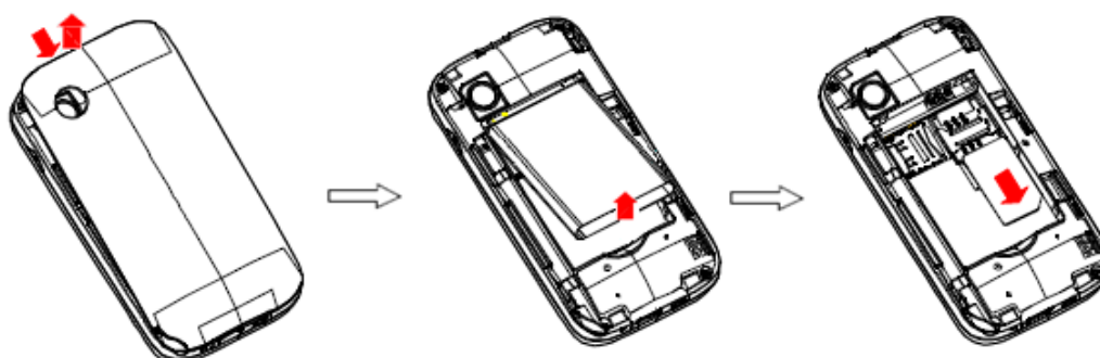
Inserting UIM card and battery
