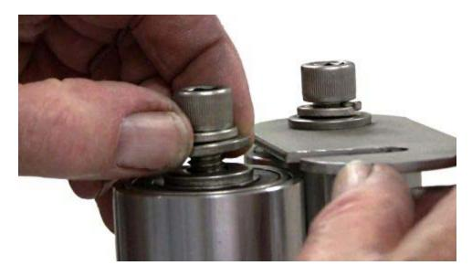
Loosen the keeper roller, move it to the top of its slot and retighten the bolt.
