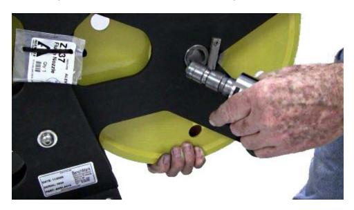
With the load pin removed gently let the tension wheel rest in the frame.
