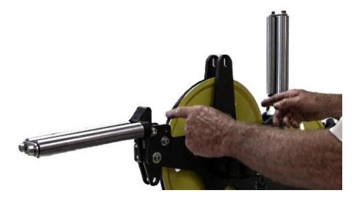
We will now remove the encoder and the wheel hubs. Remove the 4 screws holding the encoded to the adapter.
