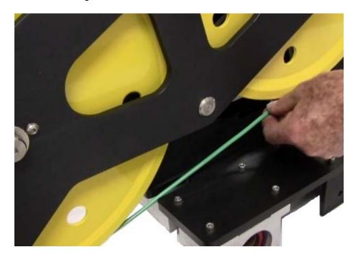
With a wrench or bar spring the pressure wheel away and thread the wire the pressure wheel and the measuring wheel.
