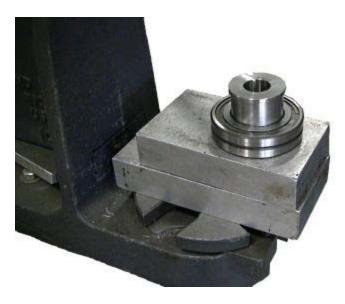
On the first stroke, the bushing may not go all the way into the bearing. Add a spacer on the bottom of the bearing as the bushing will protrude below the bottom bearing.
