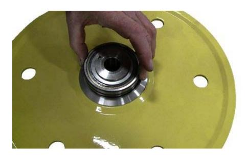
Install the 2<sup>nd</sup> snap ring to hold the bearing in place.
