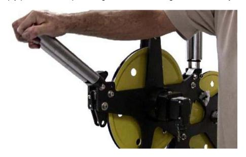
There is now clearance to remove the measuring wheel from the frame.
