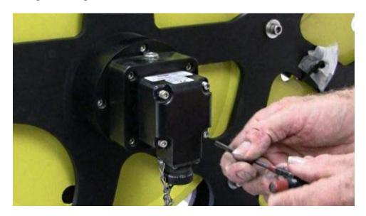
Pull the encoder straight out taking care not to jar the coupling.
