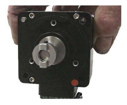
Replace the encoder while looking through the plug hole on the top and rotating the measuring wheel as necessary to get the 2 parts of the coupling to mesh.
