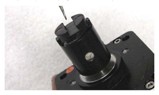
Look though the hole in the adapter body and you will see the coupling half. Rotate the measuring wheel so that the tang on the coupling half is vertical.
