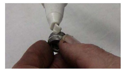
Replace the plug and tighten it firmly.
