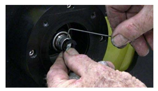
Take a wooden dowel about the size of a broom handle and put it through a hole in the measuring wheel to stop it from rotating while the large nut is removed from the shaft. Use the 1 7/16 socket and loosen and remove the nut.
