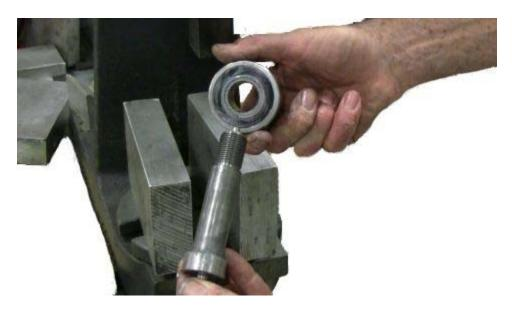
**NOTE** – make sure that the small lubrication hole on the outside bearing race is lined up with the grease fitting on the hub or the bearing won't be lubricated and will fail.
