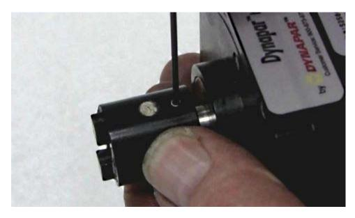
Use DC111 or equivalent and apply a thin layer to the plastic coupling. Press the plastic on top of the coupling stack. The DC111 will temporarily hold it in place.
