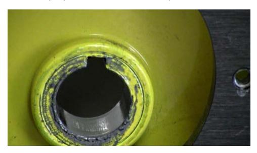
When reinstalling the shaft, rotate it so that the key goes in the keyway.
