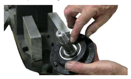
Verify that the shaft is properly aligned in the hub. If the shaft spins easily, then it is properly installed.
