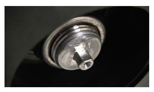
Replace the coupling on the small shaft. Align one of the set screws to the flat side of the shaft. Tighten both set screws.
