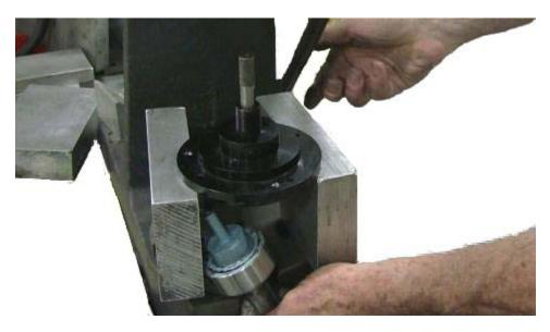
Be sure to catch the shaft – clean off any lubricant on the bearing and shaft.
