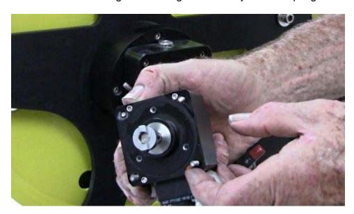
Remove the plug in the top of the adapter.
