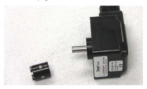
Replace the existing coupling stack on the shaft of the new encoder. Note that the shaft has a flat side. Place the coupling on the shaft so that the tangs on the coupling and one set screw are aligned to the flat side of the shaft.
