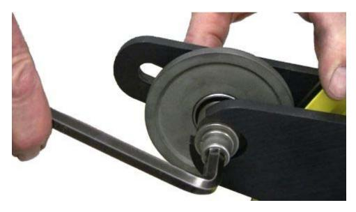
Thread the wire between the 1<sup>st</sup> set of guide rollers then over the top of the measuring wheel under the under the keeper roller.
