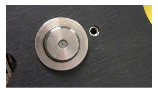
Replace the anti rotation screw and tighten it firmly.
