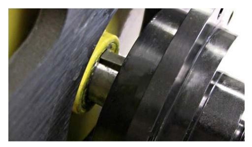
Rotate the hub so that the grease fitting faces to the right and the 4 screw holes on the hub align with the holes on the frame.
