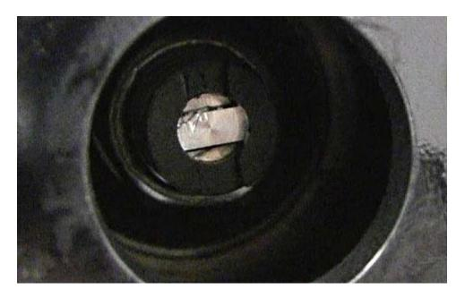
Rotate the other end of the coupler on the encoder to vertical.
