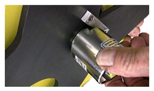
The bearing in the tension wheel has a slot for an anti rotation screw.
