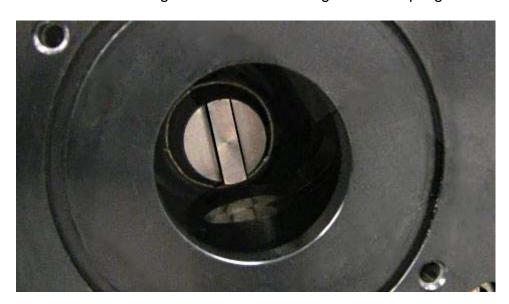
Carefully replace the encoder watching to not jar the coupling stack. Hold it against the adapter body.
