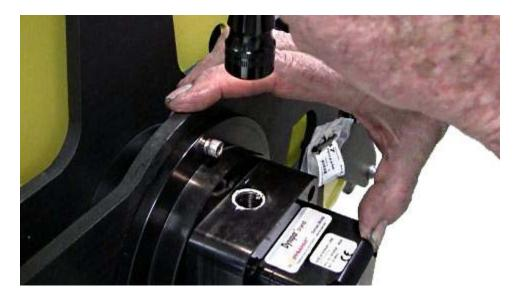
Temporarily replace the 2 screws to hold the encoder and coupling in place.
