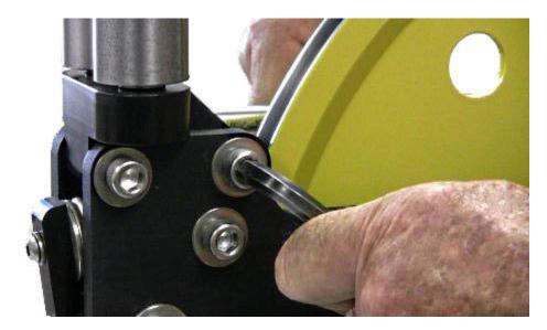
Simply push on the top of the guide roller to swing it out of the way.
