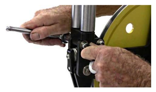
When replacing the keeper roller, make sure you have a flat washer on each side of the roller.
