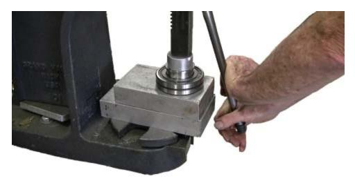
The bushing is properly installed when approximately equal amounts stick out both above and below the bearing assembly.
