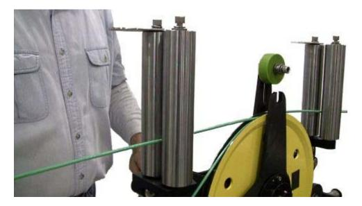
The keeper roller is now repositioned to keep the 2 rows of wires from crossing in the measuring wheel groove.
