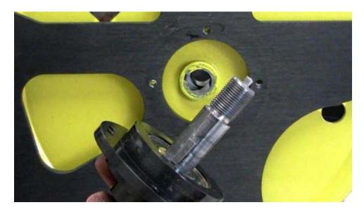
The measuring wheel is now free to be removed if necessary.
