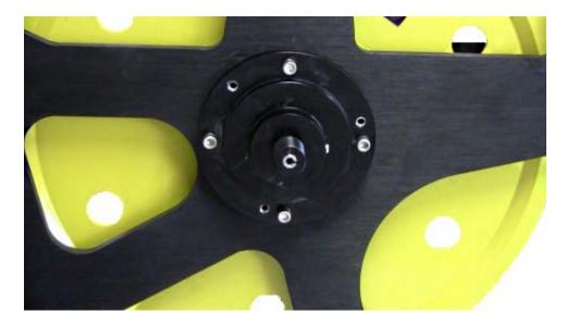
On the encoder side of the frame, if the hub was removed, you'll need to reinstall it. Rotate the hub to align the screw holes on the hub and the frame.
