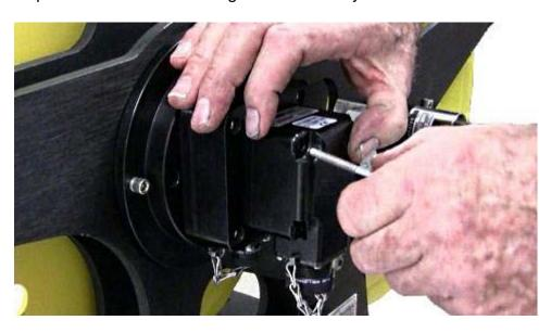
The last step in the process is to replace the plug. Put a half a bead of Teflon sealant on the leading threads of the plug.
