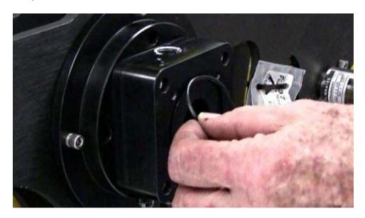
Position the coupling on the encoder so that the slot is vertical.
