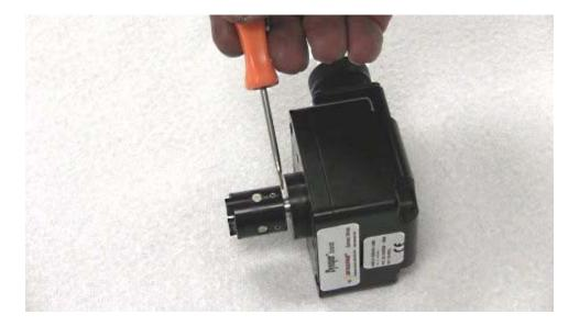
With the small Allen wrench, loosen the 2 set screws that hold the coupling on the shaft of the encoder.
