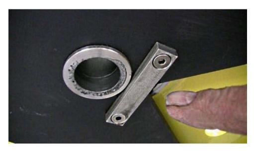
Insert the load pin and rotate it so that the flat side of the pin butts up to the guide plate.
