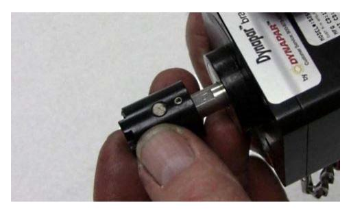
When tightening, leave the same gap on the shaft between the coupling and the encoder. Snug up but DO NOT fully tighten the set screw on the flat side of the shaft.
