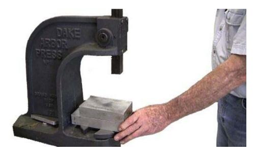
The anti-rotation bushing will be pressed into the bearing. Place the new bearing on the press.
