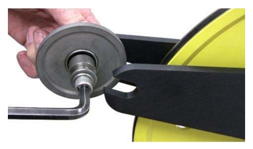
Pull the wheel up and out of the frame.
