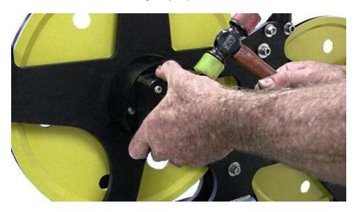
The O ring may come loose when the adapter is removed. Note the lip on the back of the adapter – it aligns with the groove on the hub.
