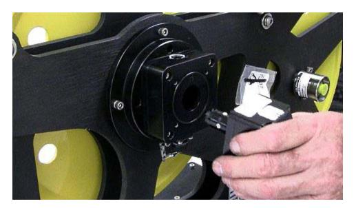
If the plastic coupling is attached to the coupling stack, remove it.
