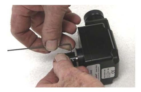
Remove the coupling stack from the shaft.
