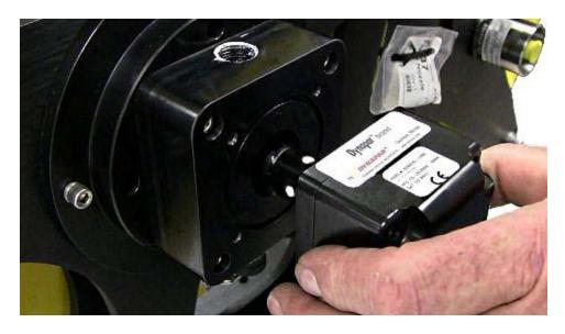
Using a flashlight look in the hole to verify that the plastic coupling has engaged the tang on the measuring wheel.
