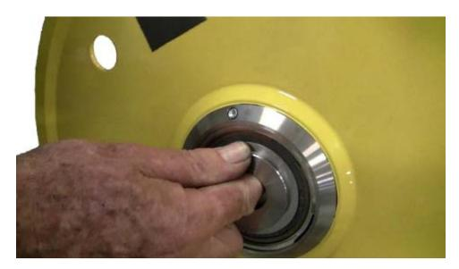
**Lubrication** – use waterproof marine grease and a straight necked grease gun. Use the grease nozzle that comes with the measuring head (in the small plastic bag zip-tied to the frame).
