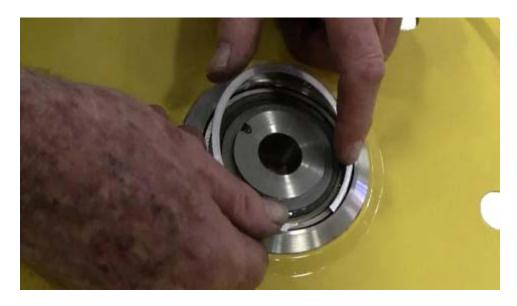
Manually tug on the bearing assembly to make sure it is firmly in place.
