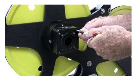
The adapter fits snugly into a recess on the hub and often needs a nudge to come loose. Use a rubber hammer and gently tap on the corner to break it loose.
