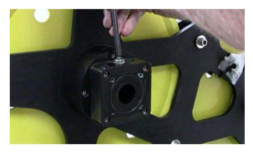
Remove the 4 screws that hold the adapter in place.
