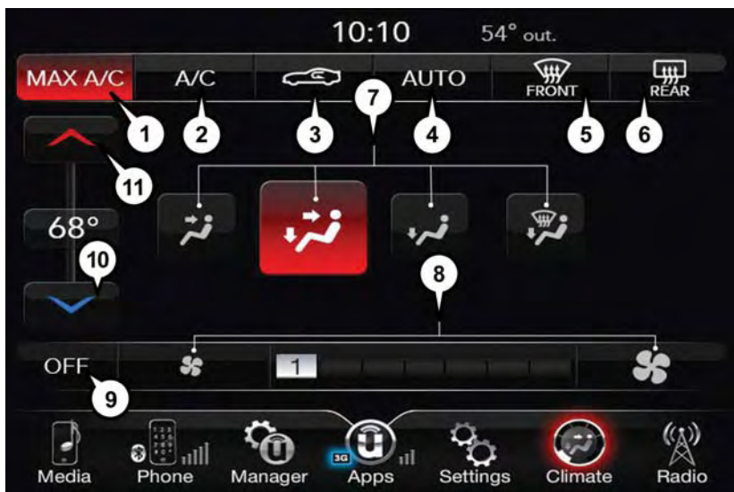
Automatic Climate Controls Touchscreen
