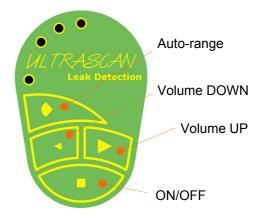
Setup is now complete and leaks can be identified by pointing the focus tube in the direction of equipment under test. Range will vary according to size and pressure of leak. A leak is indicated by flickering of the red lights (similar to volume on a HI-FI system) and is clearly audible in the earphones.
