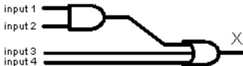
This logic function with inputs 1 and 2 AND gated results in the gate providing one input to a 3 input OR gate. If either 3 or 4 are true the output will be true. If both inputs 1 and 2 are true, the output will be true because the output of the AND gate for inputs 1 and 2 are OR gated to the result.
