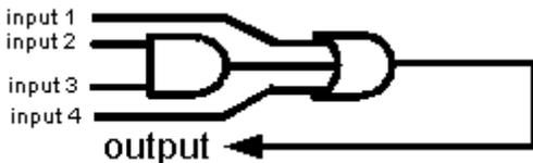
**Logical equation.**  $\text{Input 1} + (\text{Input 2} * \text{Input 3}) + \text{Input 4} = \text{Output}$
