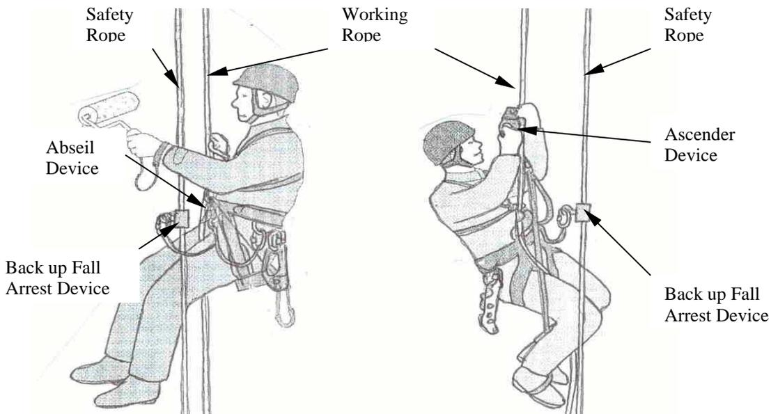
Figure 2.3.(a). Industrial Rope Access Descent. Descender device used on working rope, back-up rope grab used on safety rope.
