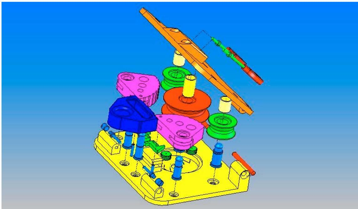
Figure 5.2. SOLIDworks Exploded View of the Back Up Fall Arrest Device Assembly
