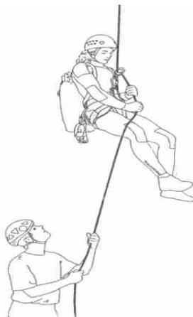
Figure 2.5. Bottom Belay Braking; an abseilers descent can be stopped/controlled by increasing the friction through the descent device by a person pulling on the free ends of the rope.
