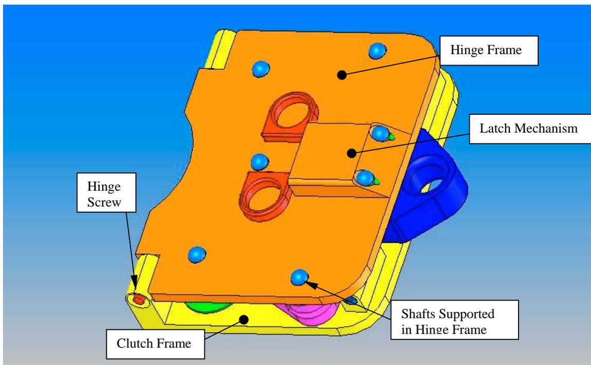
Figure 5.3. Hinge Frame in Closed and Latched Position: showing each shaft that passes through the hinge frame is supported
