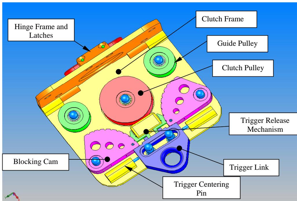
Figure 5.1. SOLIDworks Final Prototype Assembly Model of the Back Up Fall Arrest
