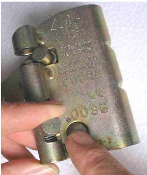
Figure 3.4.(a). Two Distinct Hand Actions Used to Unlock the “Cobra”.
