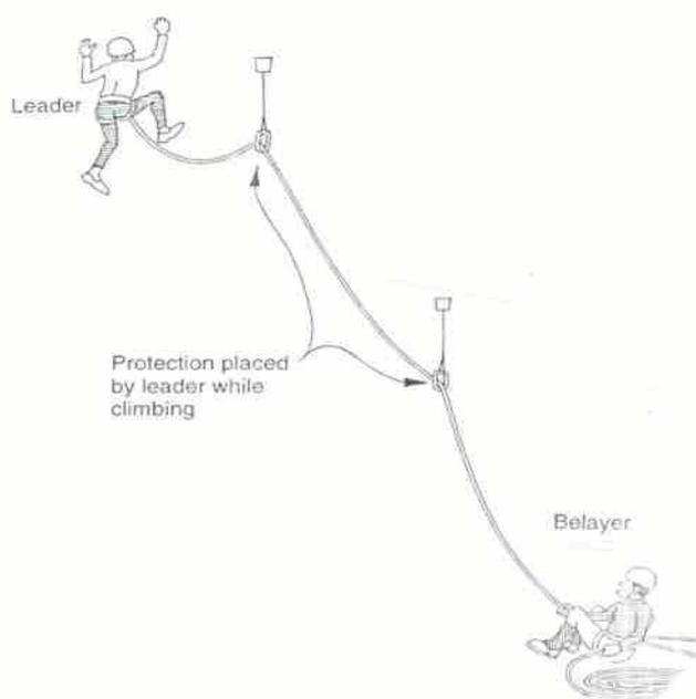
Figure 2.8. Rockclimbing Fall Arresting; climb leader being belayed by second climber
