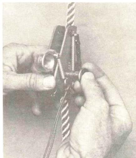
Figure 3.2.(b). Inserting the Quick Release Pin.
