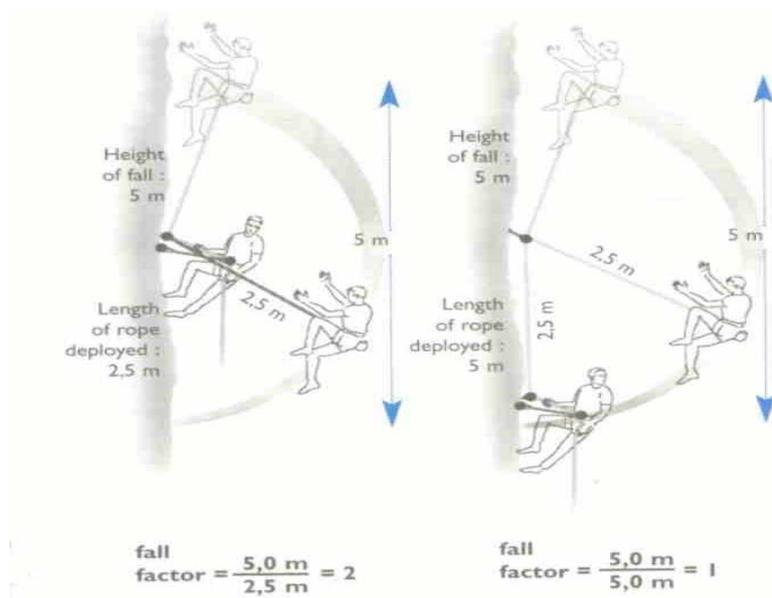
Figure 2.9.(a) The Most Severe Fall: A Factor 2 Fall
