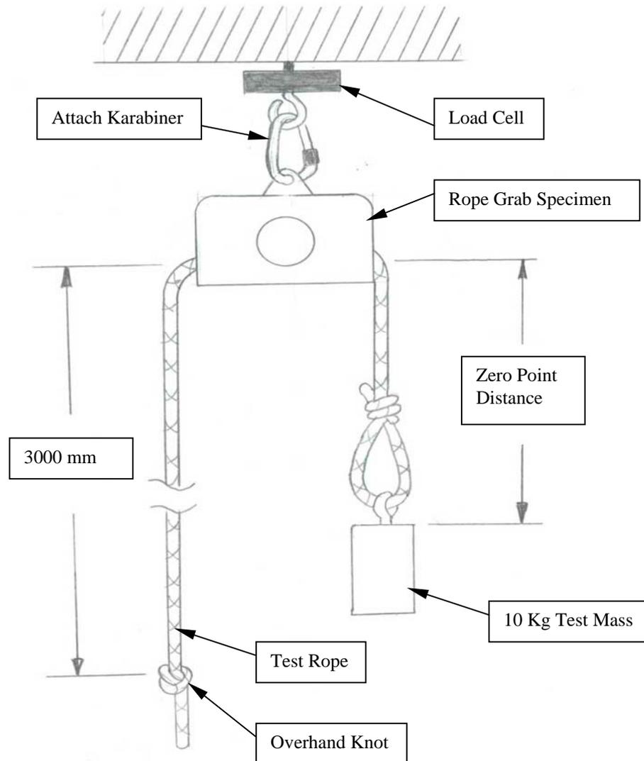
Figure 6.3. Test Set Up for the Back Up Fall Arrest Device Clutch and Cam Release Mechanism Verification Test
