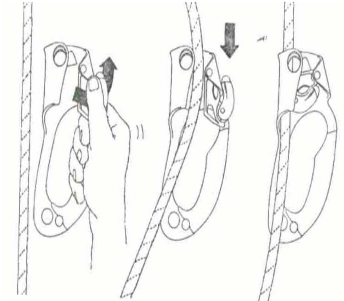
Figure 3.6.(a). Open Cam and Lock Stop on Frame Using Thumb
