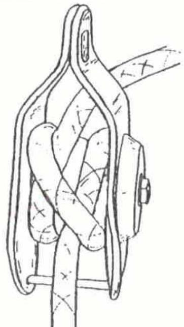
Figure 3.8.(b). The clove hitch is placed around the drum and the frame is rotated closed.
