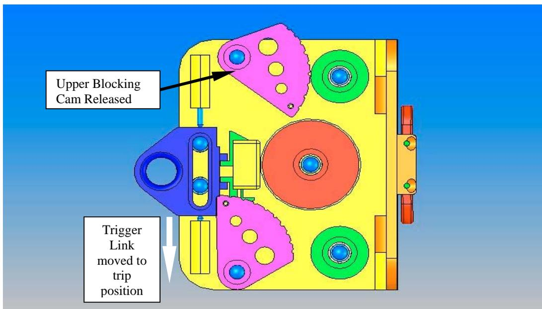
Figure 5.4. The Back Up Fall Arrest Prototype Design Shown With Trigger Link, Trigger Release Mechanism and Blocking Cam in Fall Arrest Position
