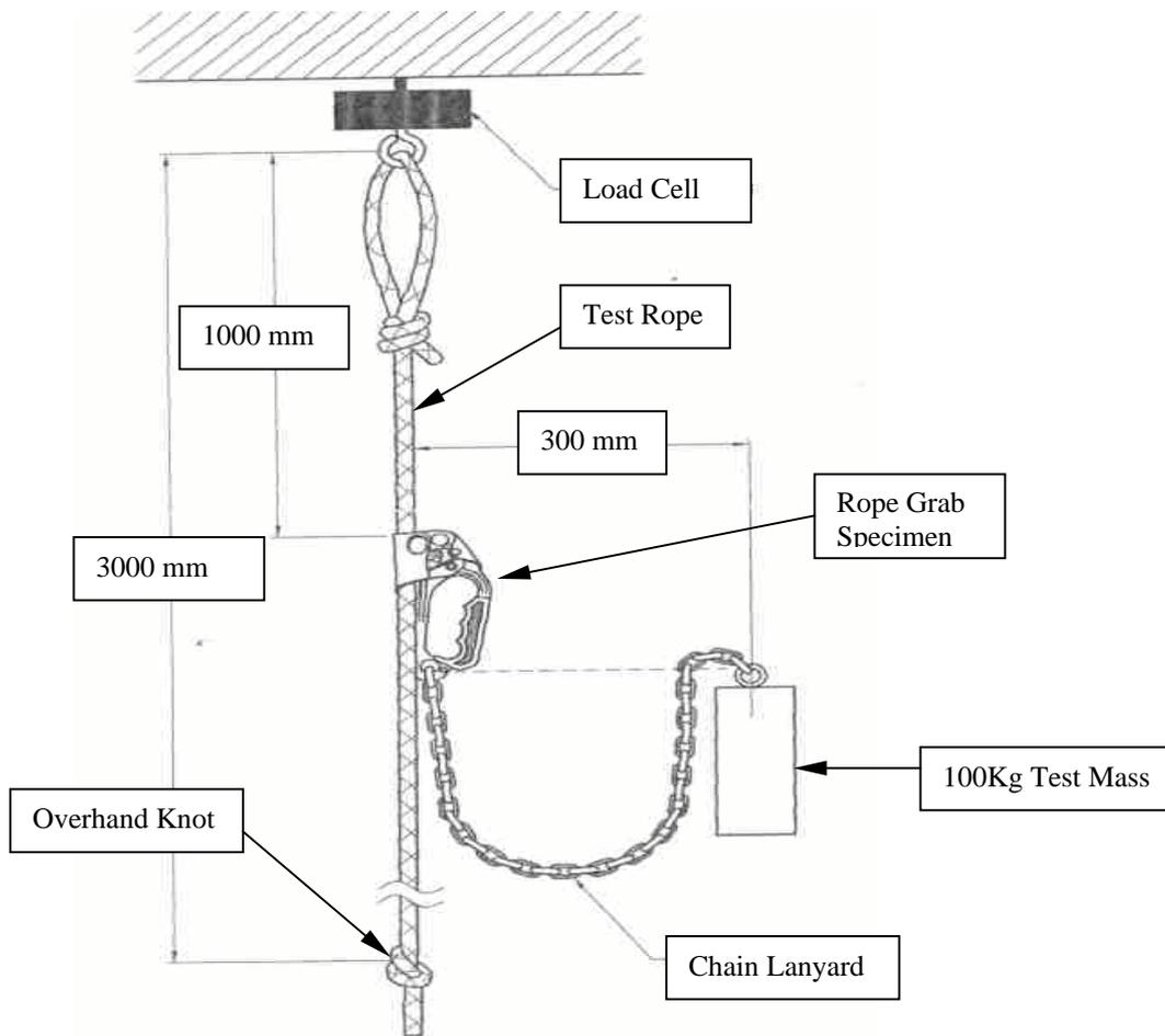
Figure 6.2. Test Set Up for Dynamic Testing of Back Up Rope-grabs as per Australia/New Zealand Standard AS/NZ4488.1:1997 Appendix B
