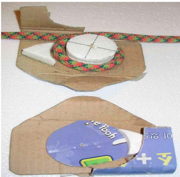
Figure 4.3. Cardboard and Polystyrene Modeling of a Rotating Frame Idea with Integral Blocking Cams on the Inertia Pulley
