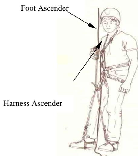
Figure 2.6. Frog Method of Ascender Rope Grab attachment; two ascenders are used – one directly attached to the cavers sit harness, the second to both feet by lanyards/cord. An alternating sit-stand position allows the caver to progressively ascend the rope.
