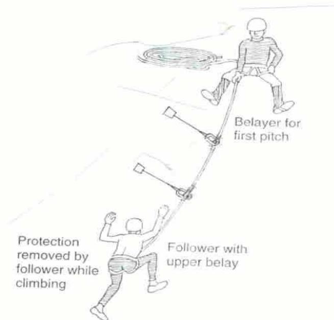
Figure 2.10. Top Rope Belay; fall protection for the second climber
