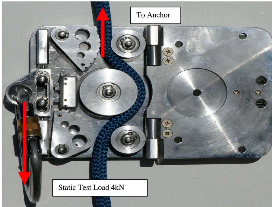
Figure 5.5. Initial Assembly of Back Up Fall Arrest Prototype Device Set Up For The Static Design Verification Test. The photograph shows:
