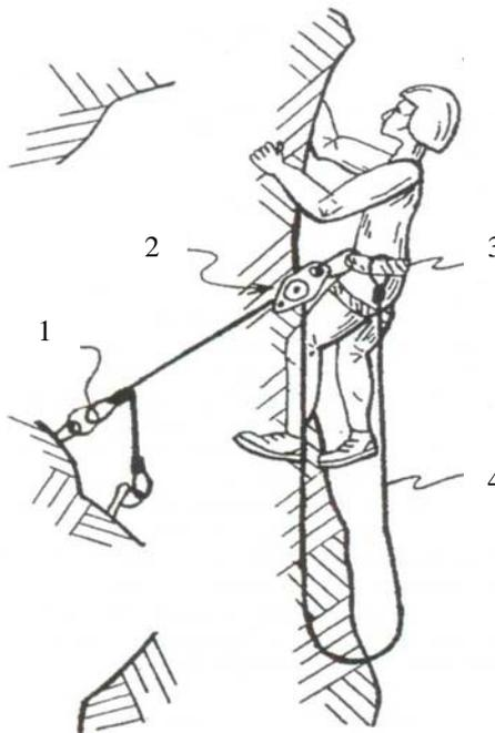
Figure 2.11 Solo Back Roped Rock Climb Showing: Anchor Point (1), Belay Device (2) Harness (3) and Belay Rope (4)
