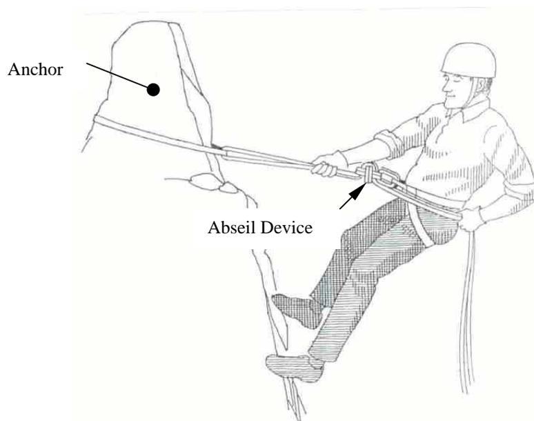
Figure 2.4. Abseiling Descent; a single or double rope is fixed to a solid anchor point, the abseiler is connected by a descender device to the rope and his harness. The abseiler can control his rate of descent by adjusting the friction through the system by increasing the load with his left-hand grip.
