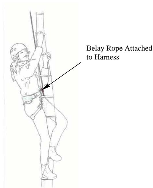
Figure 2.7. Dynamic Rope Belay of a Caver Climbing a Caving Ladder to Provide Fall Arrest.
