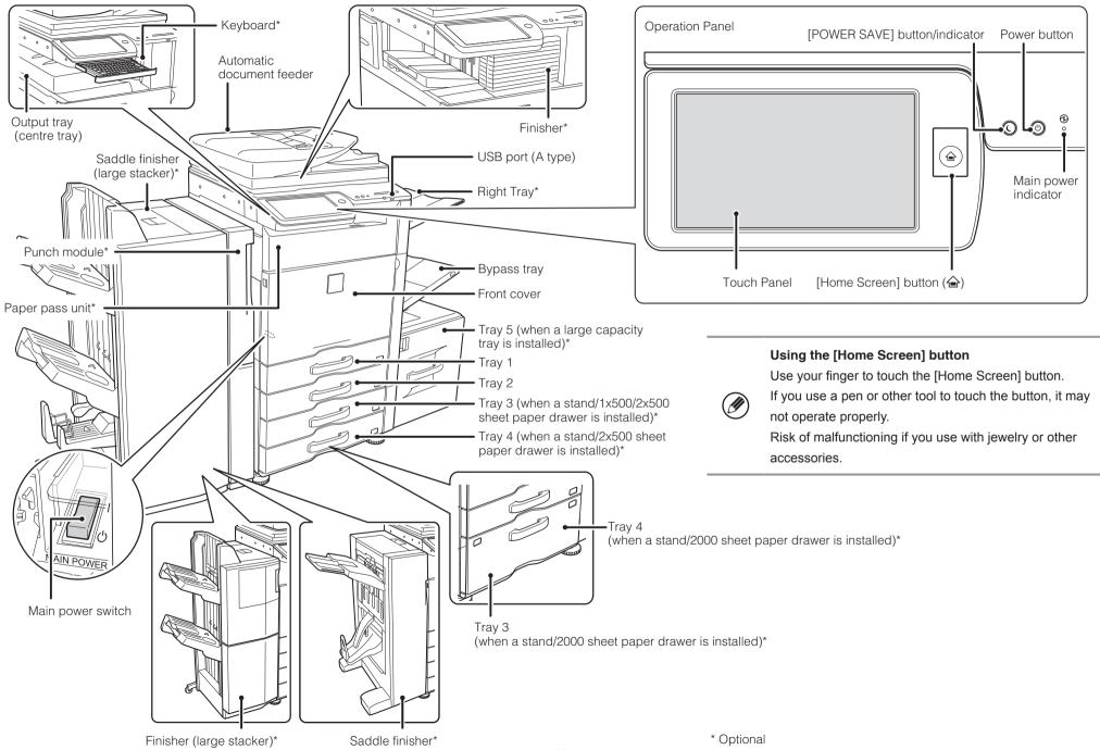
This machine has a main power switch, found at the bottom left after the front cover is opened, and a power button (()), located on the operation panel.
