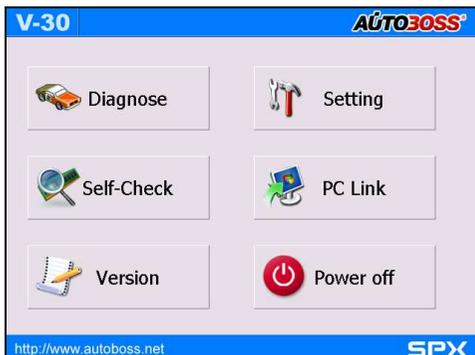
After the scanner is started, you will come to the screen shown on the left picture which includes the functions of [Diagnose], [Setting], [Self-check] and [PC link], [Version]] and [Power off].
