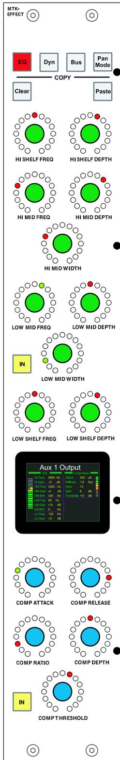
Press the **EQ**, **Dyn**, **Bus** or **Pan Mode** buttons to store the type of settings for the input channel or mix bus currently assigned to the effects panel.
