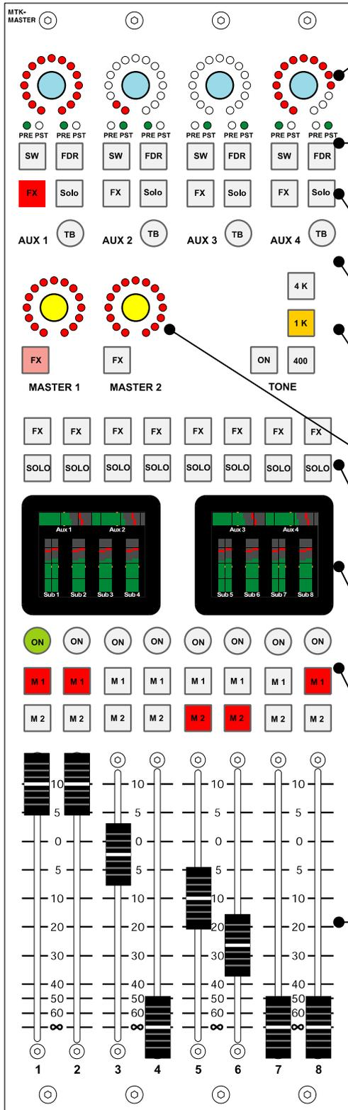
**Aux** bus master gain control for **Aux 1** through **Aux 4**. Level is indicated by *Ring of Fire* LEDs.
