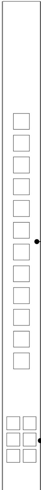
These 12 keys are programmable through *CommandBuilder*. Possible uses include control and remote record start/stop & tally. The lamps in the buttons support 16 brightness levels.
