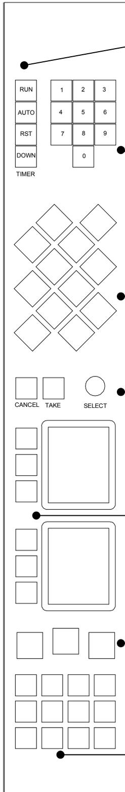
These buttons control the timer display on the **Meter Bridge** or **vScreen**. **RUN** is used to toggle the timer running. **AUTO** mode will reset the timer each time an input is turned on (where that input is not set to **Timer Disable** in *AEConfig*). **RST** will take the counter back to zero. **DOWN** will enable the number keypad to enter a countdown time.
