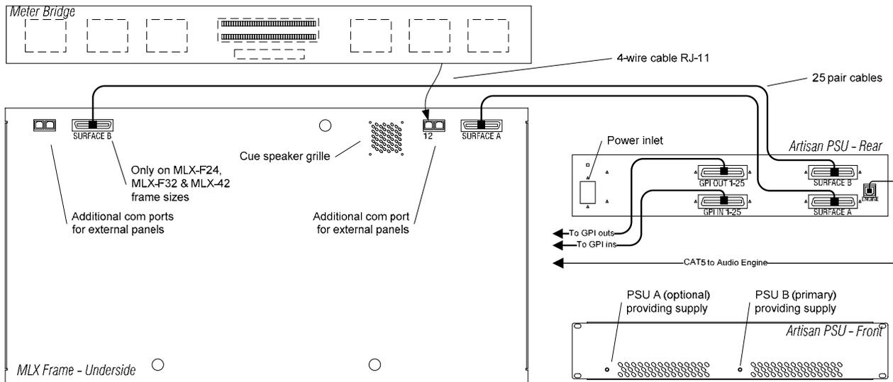
Figure 10 - Artisan Connection Diagram
