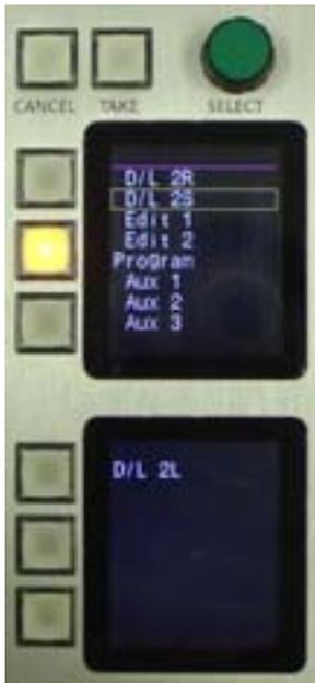
To change a **Route Select**, press the button for the destination you wish to change. The lamp will light, and a list of sources will be displayed on the top screen. Use the **SELECT** wheel to make a selection, and **TAKE** to accept the choice. Use **CANCEL** to exit the menu without making a change.
