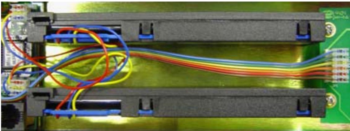
Figure 29 - Faders from underside of module
