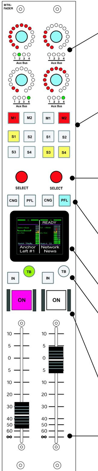
Each input can simultaneously feed any two of the four **Aux Mix** busses. Press down on an **Aux Bus** wheel to cycle between the five options; **Offline, Aux 1, Aux 2, Aux 3** or **Aux 4**.
