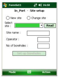
This screen fulfils two roles: it is the starting place for defining a new site, or modifying an existing one, and it provides a small number of other admin functions via the menu. The menu options are:
