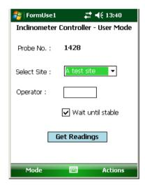
This is where the user chooses the site to be read. From the drop-down box of site names, one is selected. A three-character Operator Id can be entered if desired. If this is left blank, the Operator ID specified in the Site Setup screen will be used (the Operator ID appears in the downloaded data files). Tapping on "Get Readings" will take the user to the second User screen, where the actual readings are taken.
