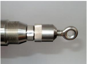
Above, the connector at the correct 'A' end of the probe for the first reading set, align the red marks prior to connection.
