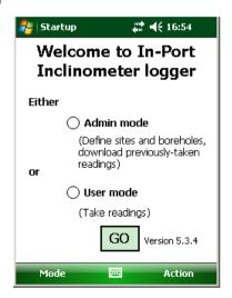
Here, the user is given the choice of which mode to work in, either by tapping the appropriate radio button and then "GO", or by choosing a mode from the "Mode" menu. As stated above, if "User" mode is chosen ensure the reel is switched on first and that approx 7-10 seconds after 'Enter Use Mode' has been selected and 'Go' pressed, that the 'comms ready' blue light on the reel illuminates.
