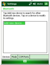
Then select "Add New Device", the Field PC will search for available Bluetooth devices and a list will appear (which may only have one device in it, the inclinometer system itself).
