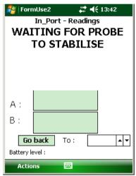
If stability checking was not chosen, the screen will immediately continue. The direction will initially be shown as "A0" and show the start depth.
