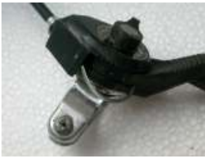
Lock lead anchor into place; Slide choke sheathing back on and hook up lever as shown
