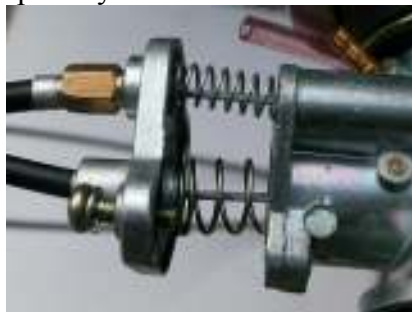
Install screws and tighten down secure making sure gasket seats correctly on carb:
