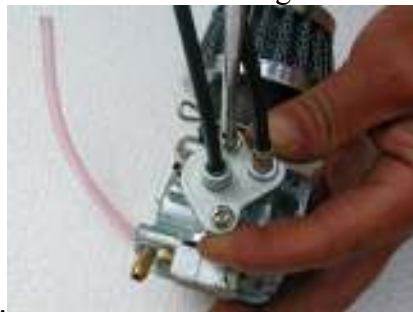
Install screws and tighten down secure making sure gasket seats correctly on carb:
