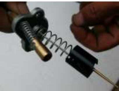
Finished hook up ready to slide back into carb. with Plastic slide slot alignment to carb. alignment
