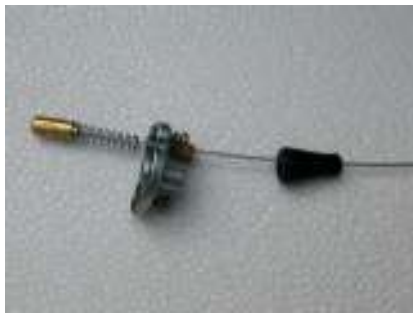
Lock lead anchor into place; Slide choke sheathing back on and hook up lever as shown
