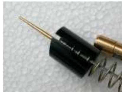
Finished hook up ready to slide back into carb. with Plastic slide slot alignment to carb. alignment
