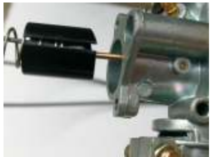
Finished hook up ready to slide back into carb. with Plastic slide slot alignment to carb. alignment
