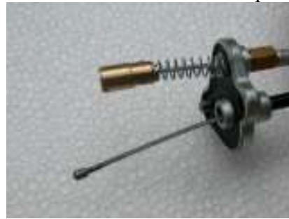
Slide throttle cable into top plate. Install big spring and collapse with fingers to hook cable anchor into plastic throttle slide then release spring.
