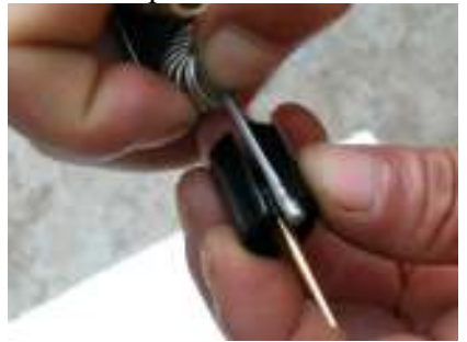
Slide throttle cable into top plate. Install big spring and collapse with fingers to hook cable anchor into plastic throttle slide then release spring.
