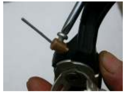
Lock lead anchor into place; Slide choke sheathing back on and hook up lever as shown
