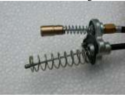
Slide throttle cable into top plate. Install big spring and collapse with fingers to hook cable anchor into plastic throttle slide then release spring.
