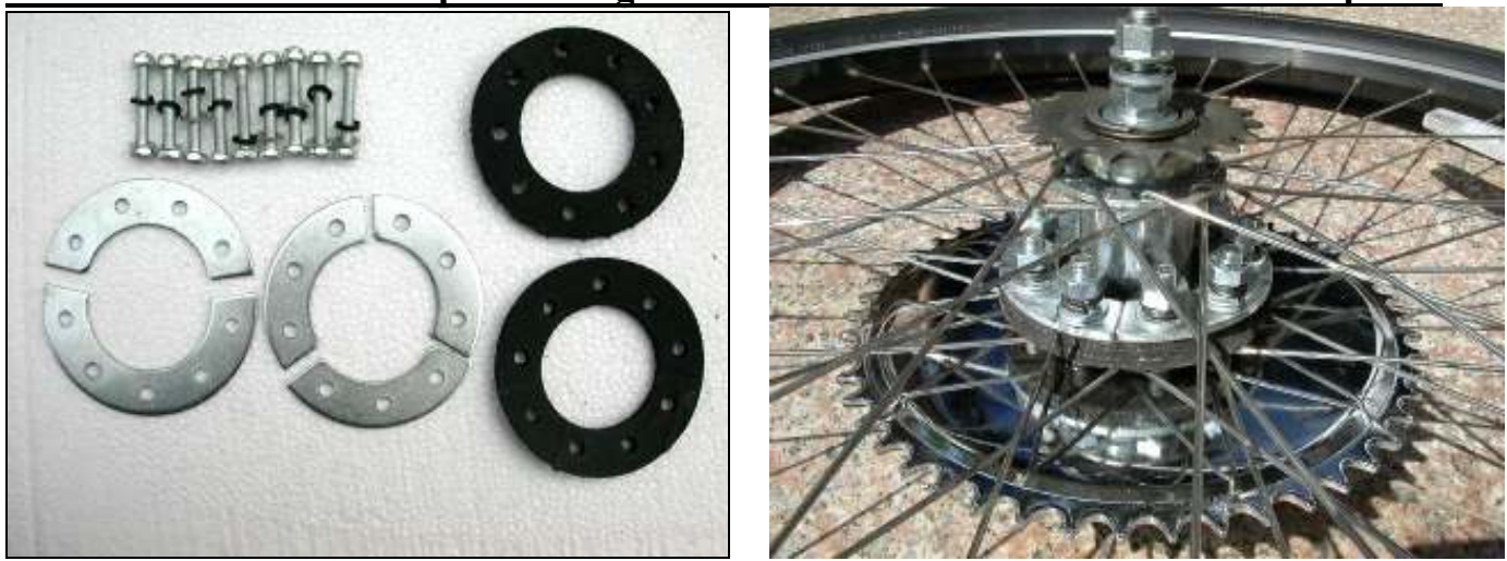
Figure #3 --- 9 hole - Chain Wheel Sprocket Installation mounted dish side inward:
