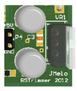
Don't ever switch polarities in the power socket, this can send your RSTrimmer directly to the recycle bin!
