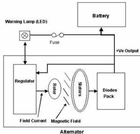
The Rotor is a coil of wire wound around an iron core. The Rotor rotates as the alternator shaft rotates and current passes through brushes. The Rotor winding passes the Field current. This causes the Rotor to produce a magnetic field. So basically the Rotor is a rotating electro magnet.
