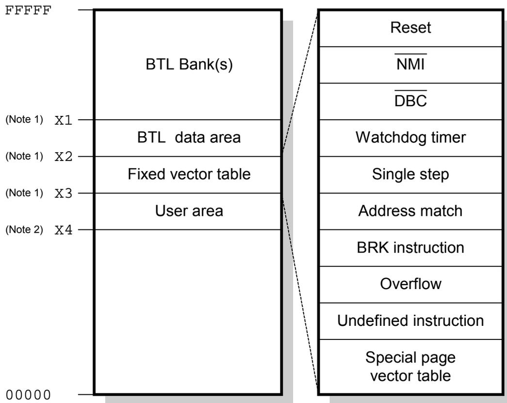
Note 1: The addresses X1-X3 depend on the target CPU. The BTL needs 8K of ROM and is located at 0xFE000-0xFFFFF. If using a target with a 16K sector at the end of the flash, the address X1 is 0xFC000. If using a target with a 8K sector or 2 4K sectors at the end, the address X1 is 0xFE000. The address X2 can be calculated as follows:  $X2 = X1 - 0x10$ . The address X3 can be calculated as follows:  $X3 = X1 - 0x34$ .
