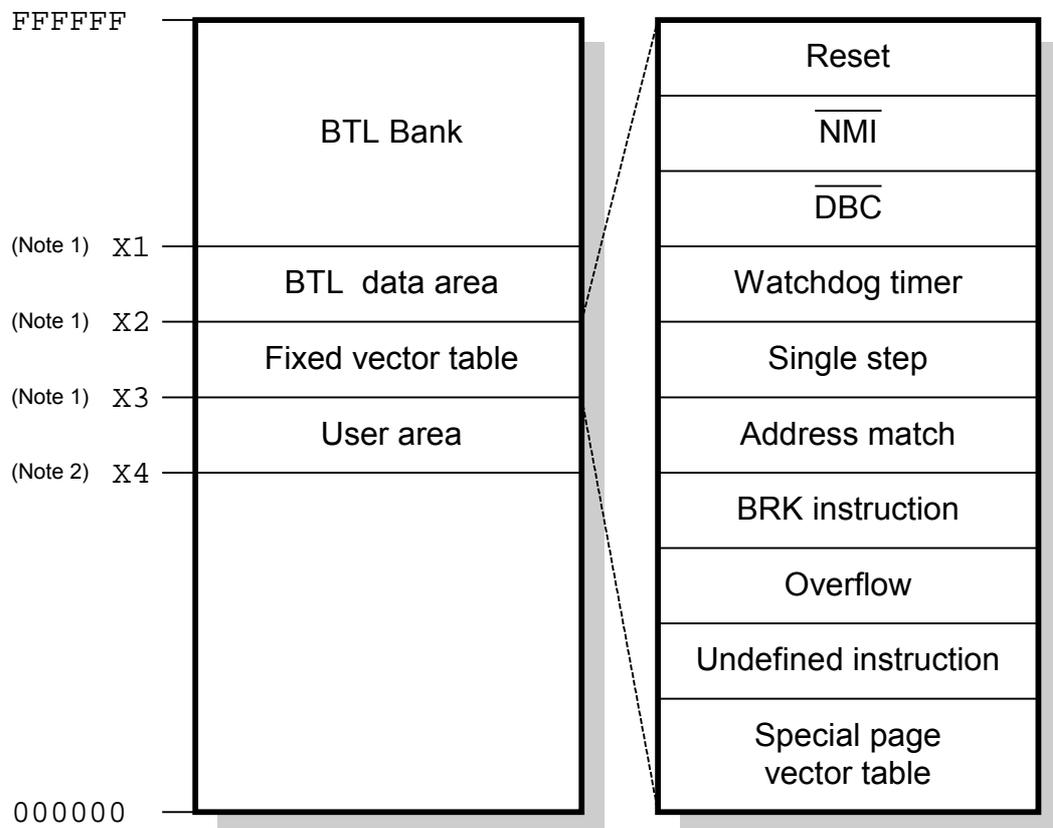
Note 1: The addresses X1-X3 depend on the target CPU. The BTL needs 4K of ROM and is located at 0xFFF000-0xFFFFF. If using a target with a 16K sector at the end of the flash, the address X1 is 0xFFC000. If using a target with a 4K sector at the end, the address X1 is 0xFFFF000. For out of the box compatibility a model for a target of 16K is shipped.
