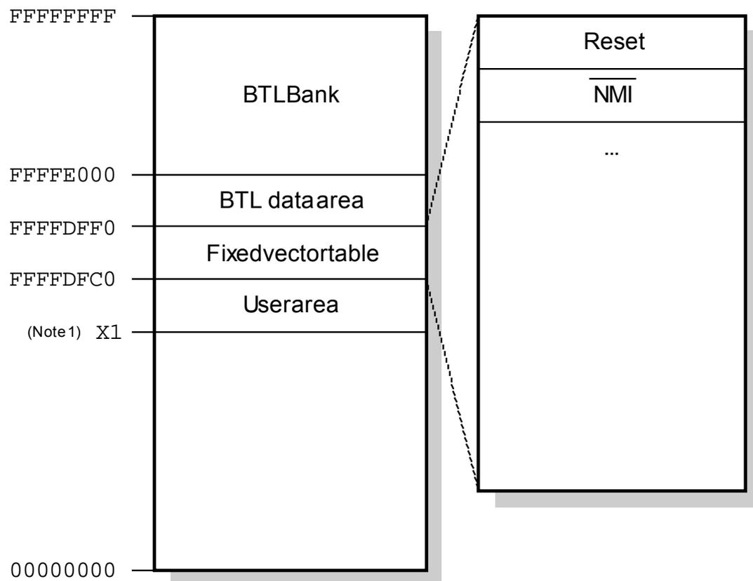
Note 1: The beginning of the user area depends on the target. The address X1 is typically the first address of the flash area, for example 0xFFFC0000 for a target with 256K of flash memory.
