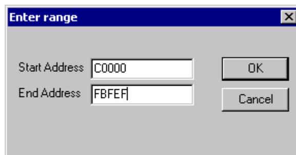
Enter start and end address and press ok to read any area of the target
