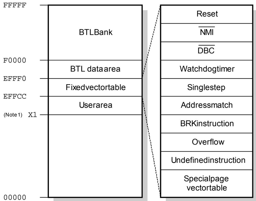
Note 1: The beginning of the user area depends on the target. The address X1 is typically the first address of the flash area, for example 0xFC000 for a target with 256K of flash memory.
