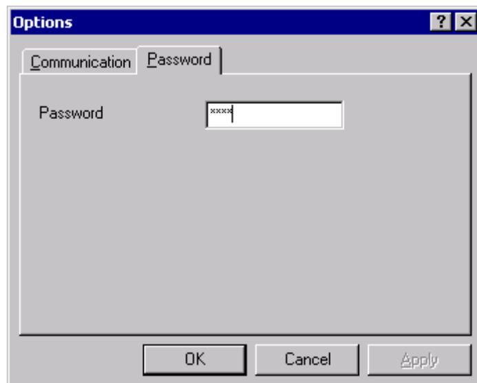
If a password is required by setting in the `Config.H` file you have to enter it here to get access to FLASH application memory area.
