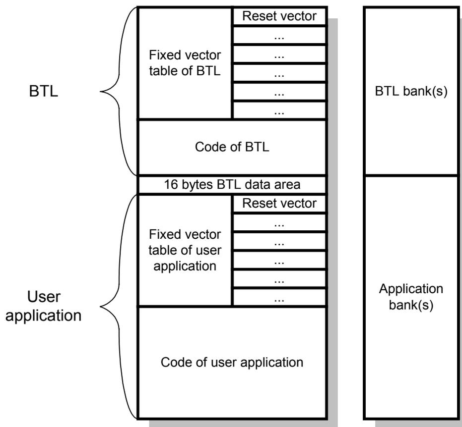
The upper 16 bytes of the user area are reserved by the BTL data area. This area typically contains the validation code which is used to tell the BTL that a valid application program is in the flash memory.
