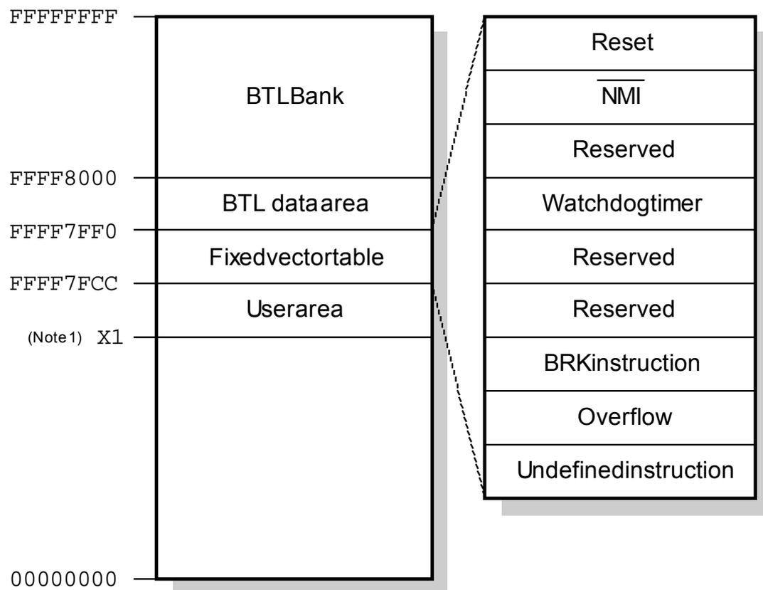
Note 1: The beginning of the user area depends on the target. The address X1 is typically the first address of the flash area, for example 0xFFFE000 for a target with 128K of flash memory.
