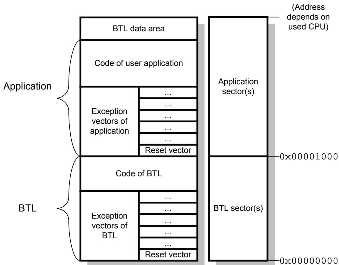
The BTL resides in the bottom sector(s) of CPUs internal FLASH. Since the RESET vector is located in this bank, the BTL is automatically started after RESET.
