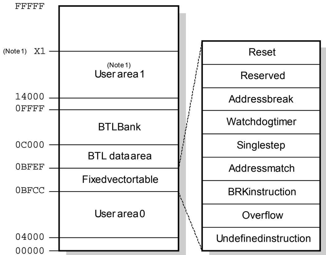
Note 1: This user area does only exist for targets with 96kByte or more flash. The end of this user area depends on the target. The address X1 is typically the last address of the flash blocks after the flash block containing the BTL, for example 0x23FFF for a target with 128kByte of flash memory.
