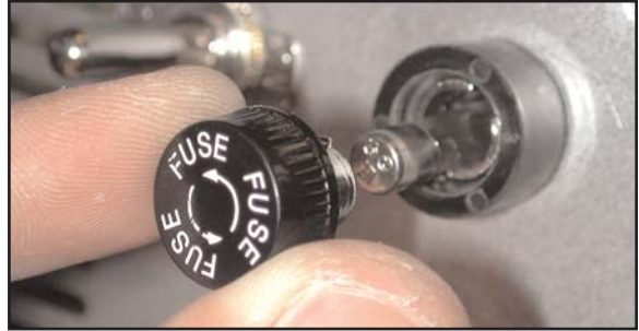
Picture of the on/off switch and fuse holder opened.
