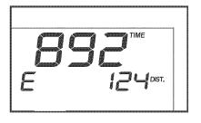
total number of miles or kilometers that the walking belt has moved. An "E" for English miles or an "M" for metric kilometers will appear in the lower left corner of the display. Press the Speed increase button to change the unit of measurement if desired. **IMPORTANT:** If a "d" appears in the lower left corner of the display, the console is in the "demo" mode. This mode is intended to be used only when a treadmill is dis-
