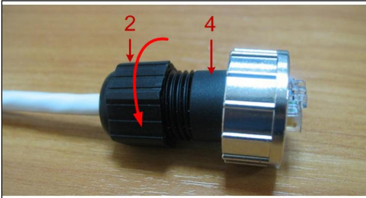
Step 5. Screw Part 2 on Part 4. This fixes the "RJ-45" connector on the cable. Check that the connector is properly fixed on the cable.
