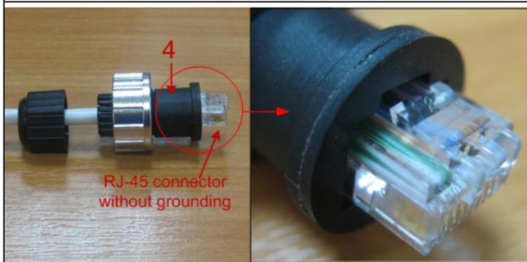
Step 4. Put Part 4 on the attached in the previous step RJ-45 connector.
