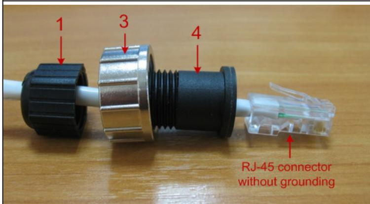
Step 3. Put connector parts on the STP service cable as shown.
