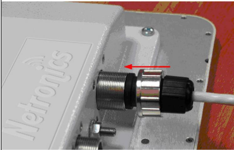
Step 6. Assemble the connector to the unit.
