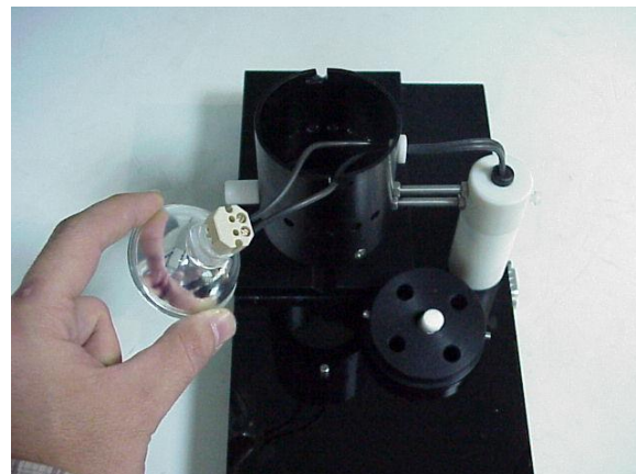
Figure 11. Unscrew the wires and change the lamp.
