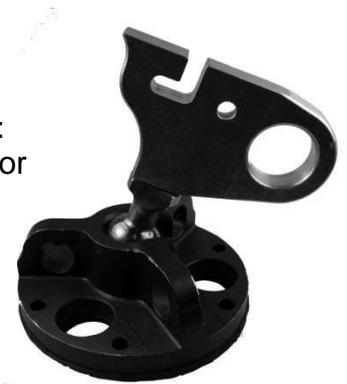
If the angle between the leg and the surface does not allow the base of the articulating foot to rest flat on the surface, the base needs to be rotated to align the notch which allows the base to rest flat on the surface. If the base does not rest completely flat against the surface, relatively light loads will damage the ball socket joint and/or could cause complete failure of the socket joint resulting in the base being detached from the TerrAdaptor.
