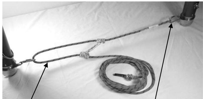
Fig 12 Rope Hobble Loop with Prussic. Sewn loop connected to quick link; large loop connected to 2<sup>nd</sup> leg quick link.
