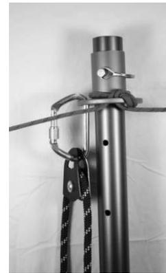
Fig 23 Lash Ring atop of gin pole as main attachment
