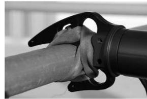
Spikes can be sharpened with a hand file or replaced as they wear. To replace spikes, loosen the small set screws on the side of the Talon points and with hand pliers pull the spikes out from the end. Install new spikes and then tighten the set screws.
