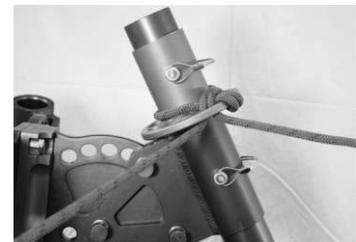
**Fig 21 Lash ring on tripod**
