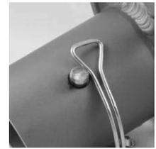
Fig 3 Improperly Secured Leg Coupling Pin
