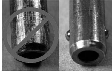
Fig 16 Left pin – retired due to wear and detent pins not properly working;
