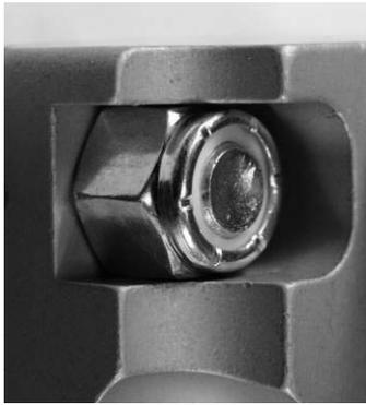
**Fig 19 Bolt protrudes just beyond flush**
