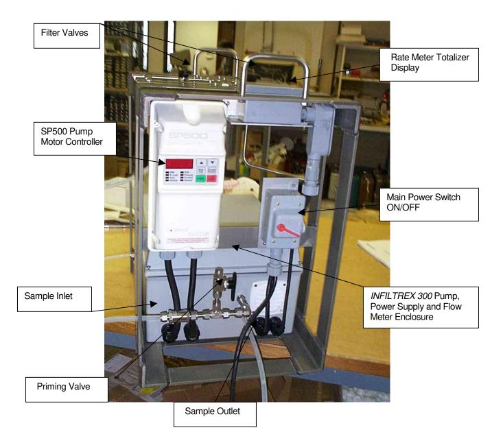
Figure 1. Side View of the INFILTREX 300 Sampling System
