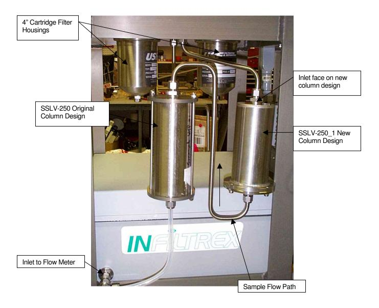
Figure 2. Front View of the INFILTREX 300 Sampling System
