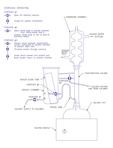
Figure 5. Soxhlet Apparatus for the Cleaning of XAD-2 Resin.
