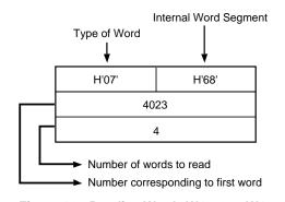
Figure 13: Reading Words W4023 to W4026: Transmission Text Block
