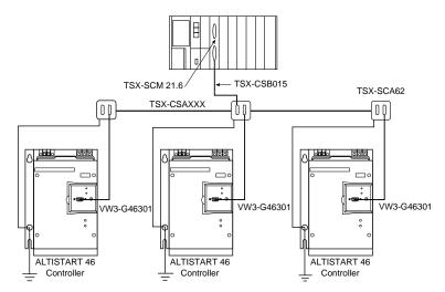
Figure 8: Example of Connection to UNI-TELWAY Bus
