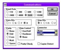
NOTE: When you select the parity bit, the number of data bits changes to 7. In this case, change the number of stop bits to 2 to restore the number of data bits to 8. Then set the number of stop bits back to 1. Saving the terminal configuration to a \*.trm file is recommended.
