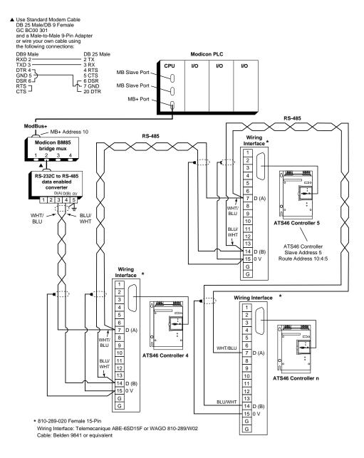
Figure 9: MODBUS Network Diagram
