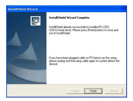
Now plug ACT-IR100UD-v2 into USB port. System will pop up a "Found New Hardware" bubble window at the right corner of Tool Bar and display the message: "Prolific USB-to-Serial Comm Port" the first time you plug in.
