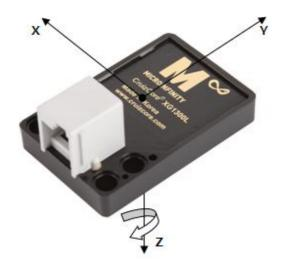
Figure 1: The CruizCore XGL1300L sensor reference frame
