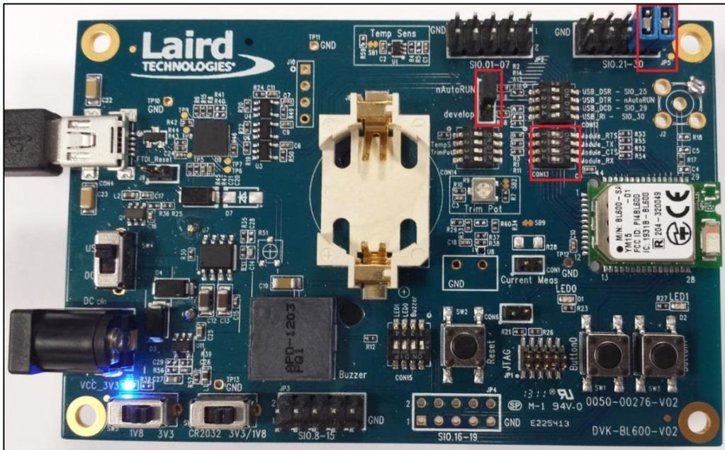
Figure 11: Host less autorun configuration
