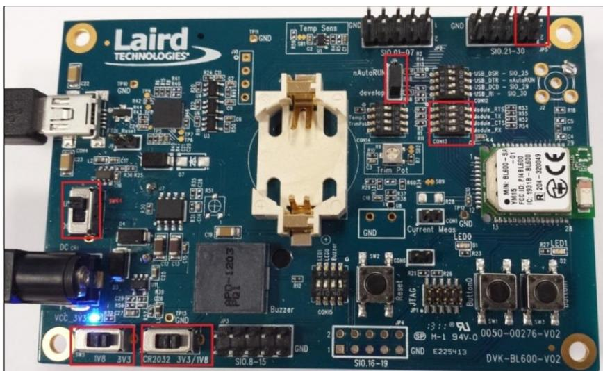
Figure 2: Switch and jumpers position
