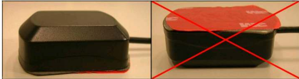
Pic. 1. GPS antenna correct mounting
