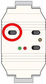
Figure 2: Switch for High-speed CAN termination
