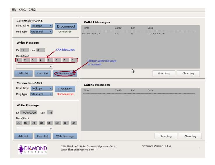
To transmit to a different CAN ID, change the data in the CAN ID field, enter the desired data into the Data (Hex) fields, and click on "Write Message".
