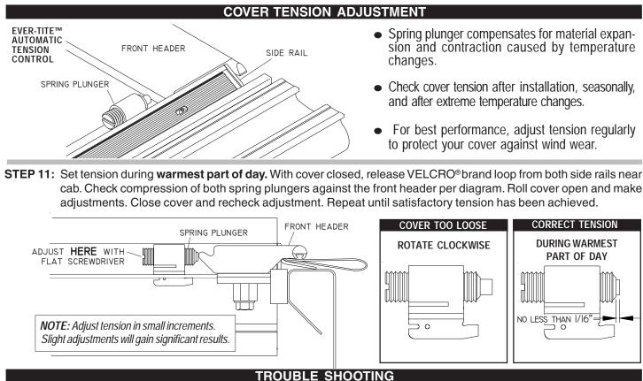
**HEADER WILL NOT LATCH:** Make sure the header seal is not caught between side rail and header. FABRIC COVER IS TOO TIGHT OR TOO LOOSE: See Step 11 to adjust tension.
