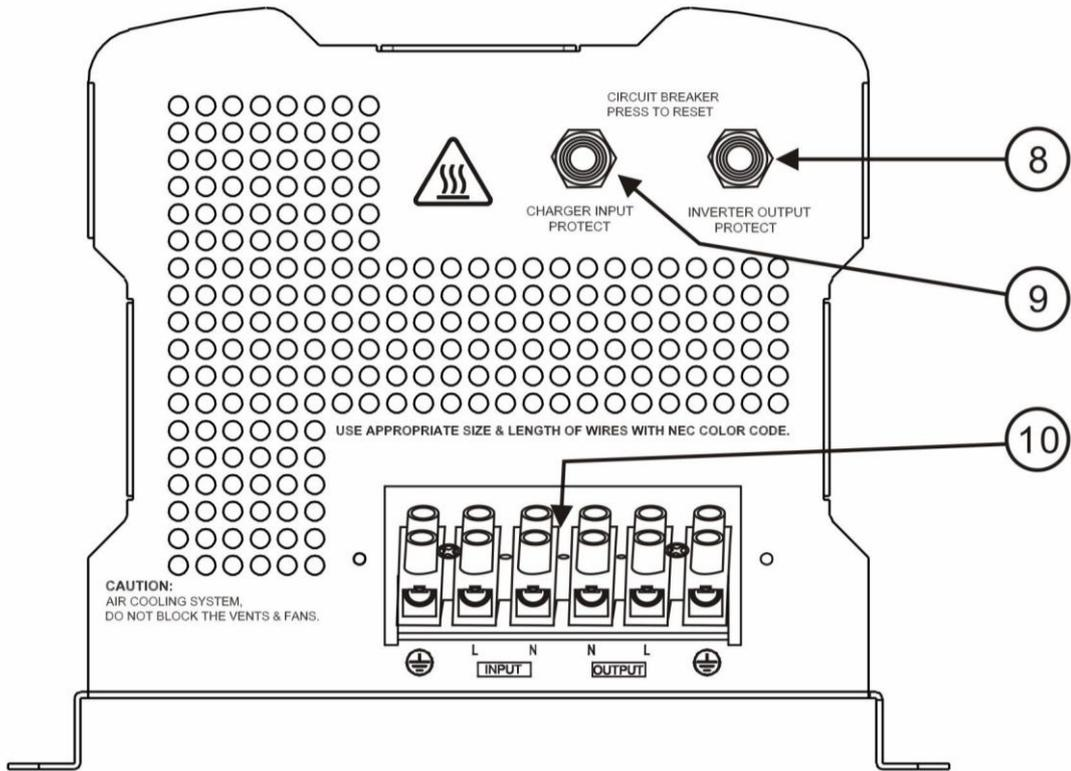
**AC SIDE FOR TXF Series 4KW to 6KW Models**
