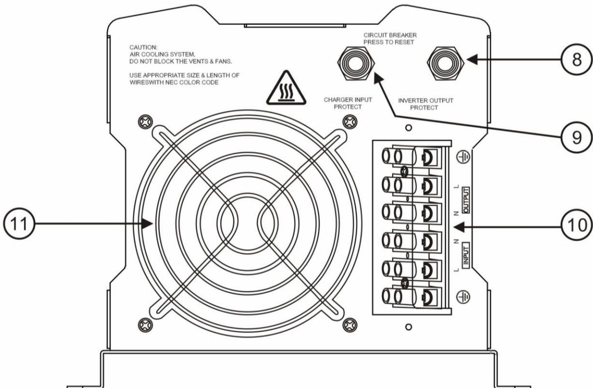
**8 Inverter Output Protection Circuit Breaker**
