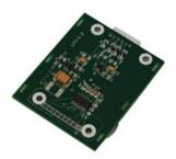
Fully digital circuit design with *light-frequency-conversion* sensor makes the oximetry modules more sensitive and accurate at low perfusion, more reliable and smaller in size.
