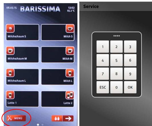
The Customer menu is protected by a PIN (Personal Identification Number). To access this PIN-protected level "XXXXXX" must be entered.
