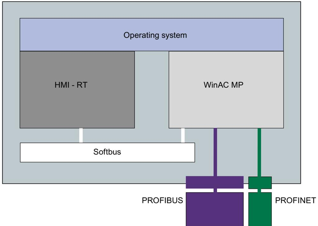
Routing from Ethernet to PROFIBUS DP with WinAC MP
