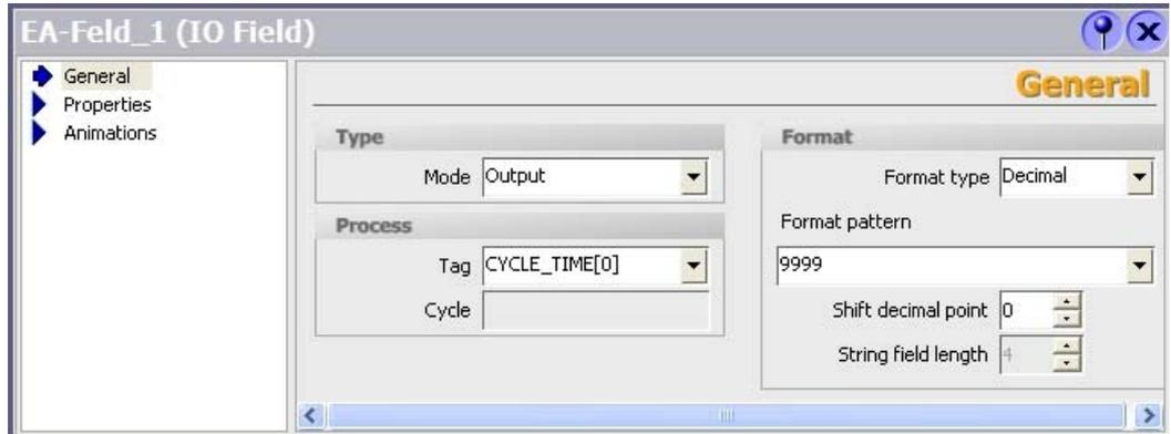
2. In the same way, assign the elements of the array variable CYCLE\_TIME to the remaining 6 IO fields. Make sure that the CYCLE\_TIME variable is incremented by 1 in each case.
