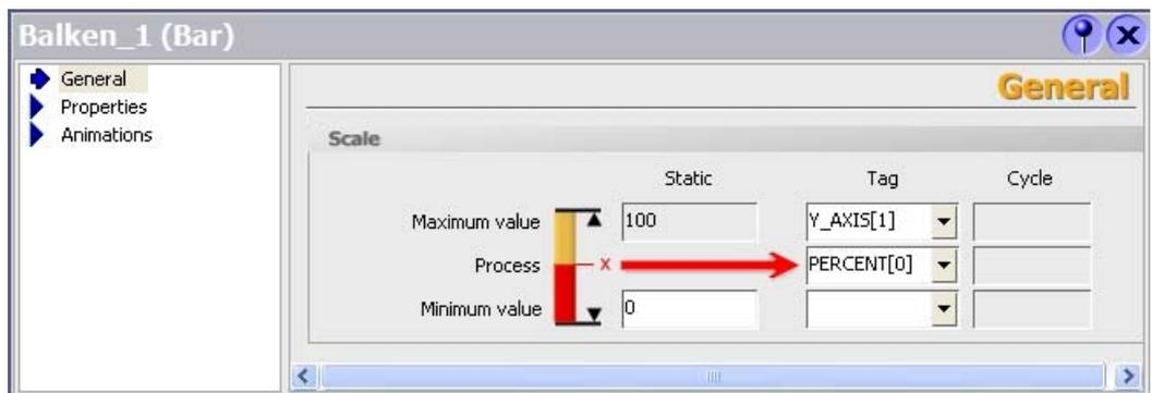
4. Click on the first bar in the histogram (Bar\_2) and assign the variables based on the following figure:
