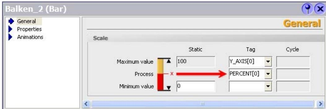
5. In the same way, assign the tags to the remaining 6 bars. Make sure that each element of the PERCENT array variable is incremented by the count of 1.
