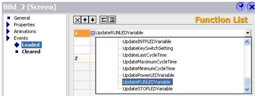
9. For the parameter "RUN: (output)" of the "UpdateRUNLEDVariable" function, configure the internal variable "RUNLED" of the data type INT.
