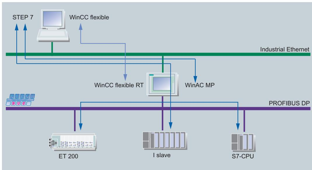
Figure 4-4 Routing from Ethernet to PROFIBUS DP with WinAC MP
