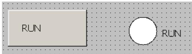
4. Assign a switching function to the RUN button: Select the RUN button and click on **Events > Click** in the lower area of WinCC flexible.
