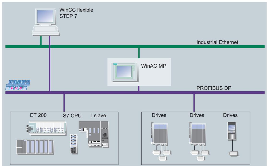
Figure 2-1 Embedded automation with WinAC MP 2008
