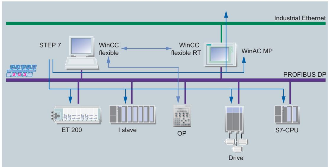
Figure 4-5 Routing with WinAC MP over PROFIBUS
