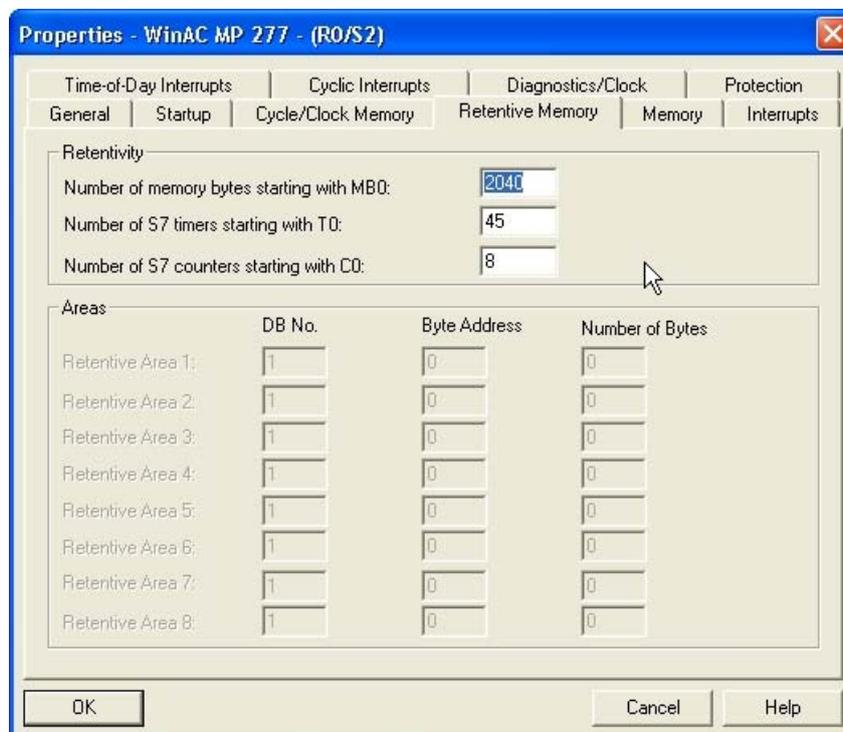
Figure 4-1 Properties of memory bytes, S7 timers, S7 counters
