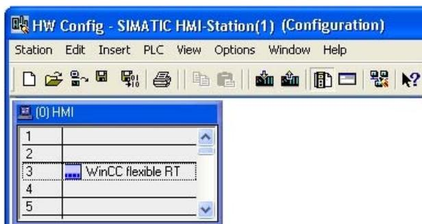
7. In the hardware catalog, go to the SIMATIC HMI Station > Controller > WinAC MP folder and, depending on the Multi Panel selected under item 3, select:
