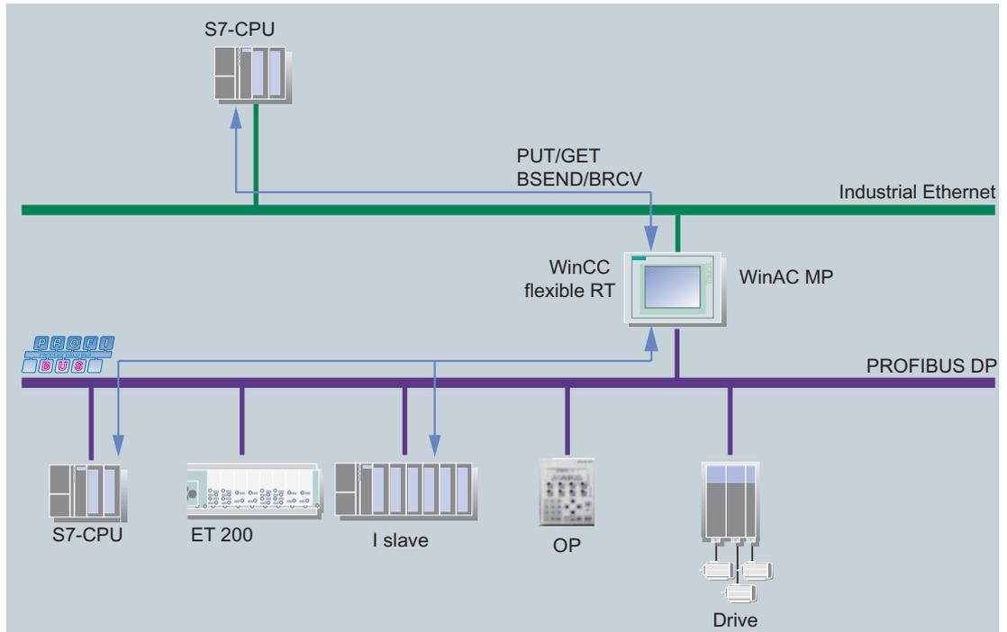
Figure 4-7 CPU-CPU communication over WinAC MP
