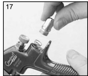
17. Replace Valve Spring and screw in Housing (10).
