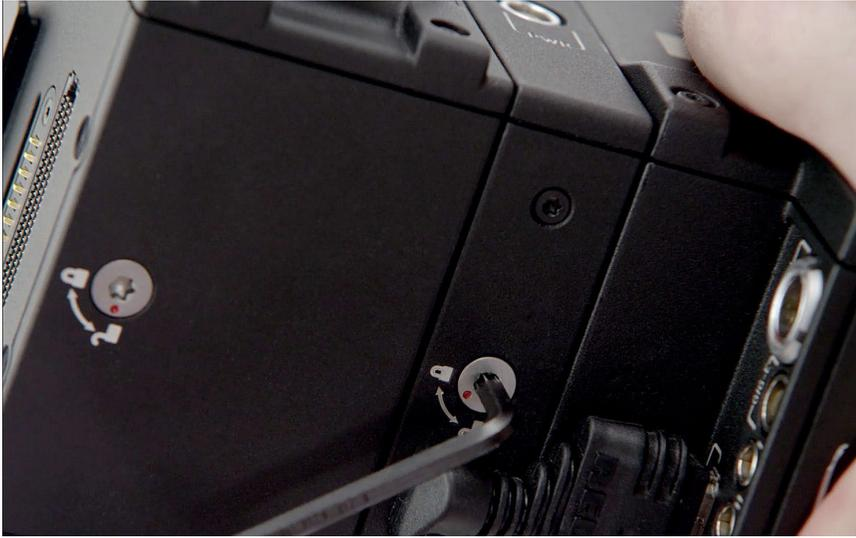
The REDCAST Module is secured.
