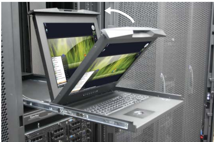
Figure 5. Flipping up the LCD to a suitable angle.
