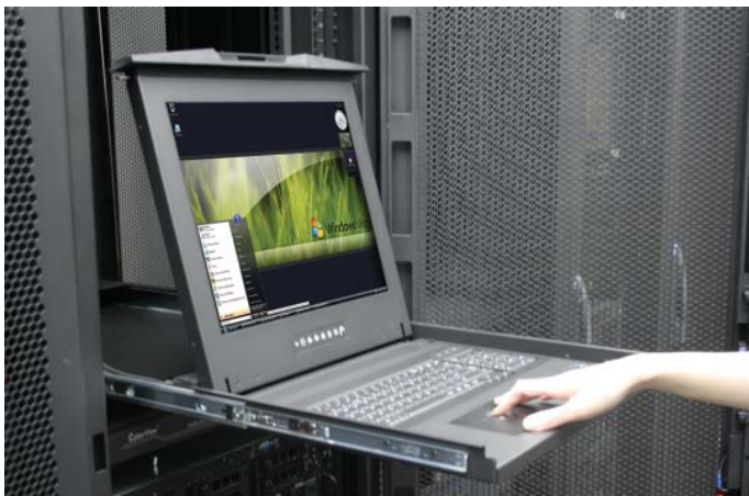
Figure 6. Operating the LCD keyboard drawer.
