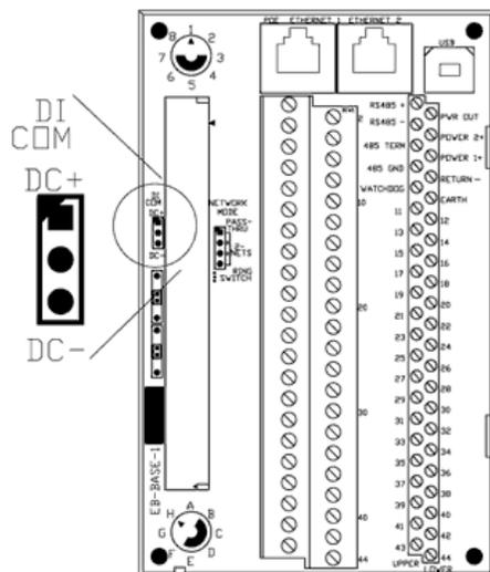
NOTE: The DI COM jumper is located on the base so that the replacement of a module or inadvertent change in configuration from the web server or I/O Tool Kit software will not adversely affect the power wiring on the affected inputs.
