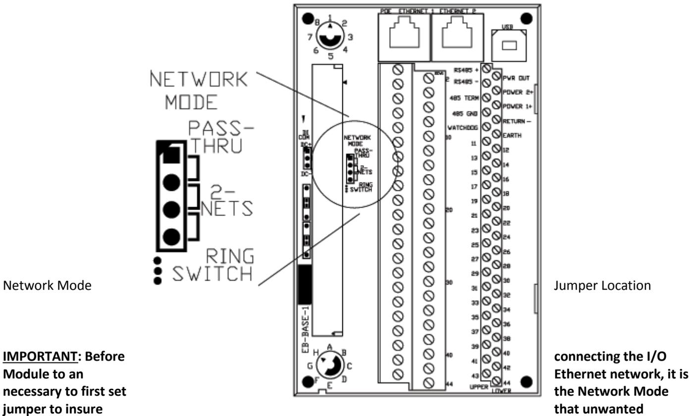
NOTE: The jumper is located on the base so that the replacement of a module or inadvertent change in configuration will not adversely affect the network.
