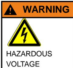
**If damage can be seen on the faceplate of the Dialog-Controller, the device must not be operated any more! It must be disconnected from the supply voltage immediately!**
