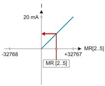
When a current range has been configured, the JX3-AO4 module converts - in linear mode - a digital value into a current. Conversion is carried out according to the following formula:
