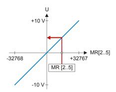
When a voltage range has been configured, the JX3-AO4 module converts a digital value in linear mode into a voltage. Conversion is carried out according to the following formula:
