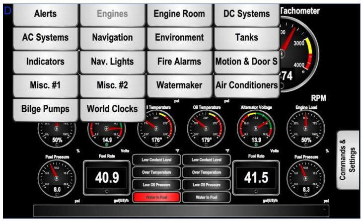
Figure 10 – N2KView® Window with Tabs Displayed
