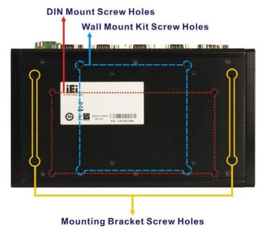
Figure 2 - Mounting Bracket Screw Hole Locations
